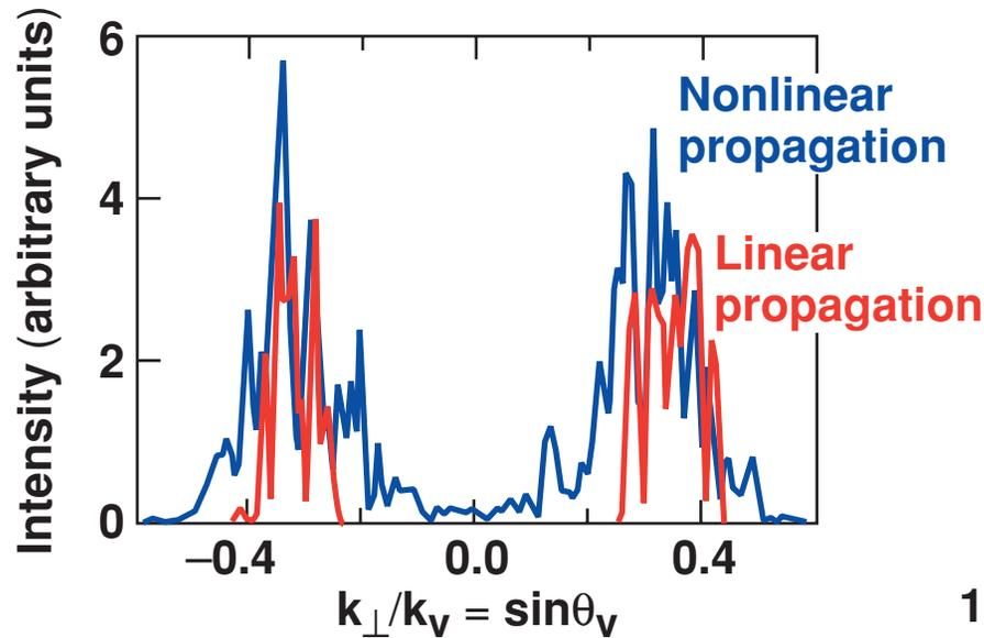
Two DPP beams with average intensity  $\langle I \rangle_{14} = 7$  in each beam and angle of incidence  $\pm 20^\circ$
