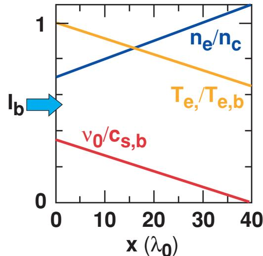
Profiles of density, flow, and temperature modeling OMEGA plasma near critical density (similar to simulations by *SAGE*).
