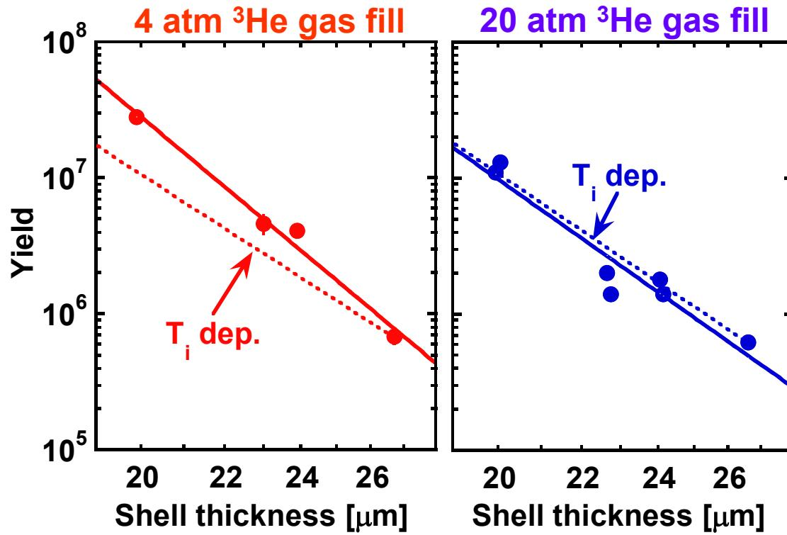
Similar levels of mix are observed for 27-μm thick shells irrespective fill pressure.
