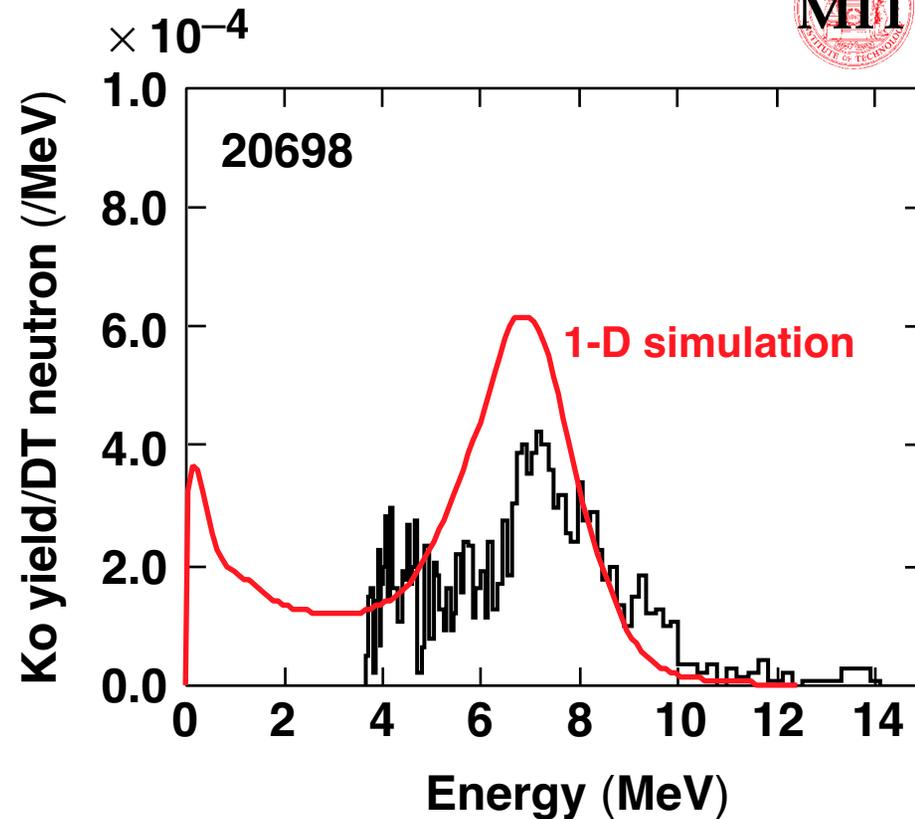
$\rho R$  (expt)  $\sim 13 \text{ mg/cm}^2$ ;  $\rho R$  (1-D)  $\sim 17 \text{ mg/cm}^2$ .
