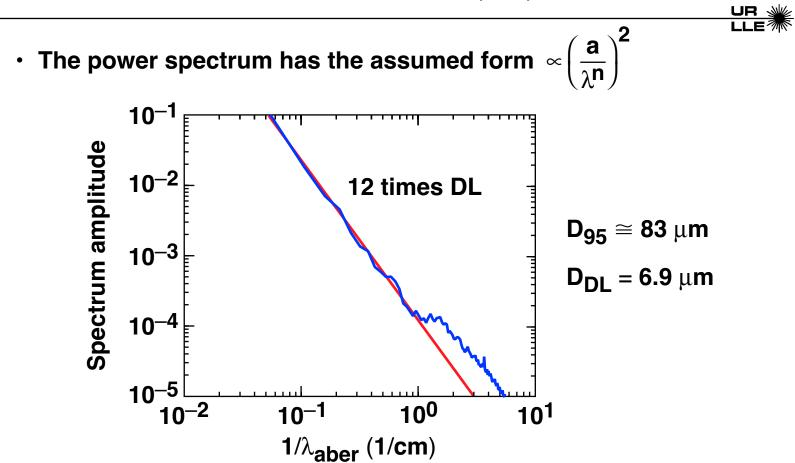
• The amplitude a is varied, and the strength of the aberration is measured in terms of times diffraction limited:
