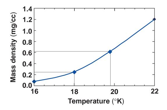
**Operating at the triple point almost triples the mass density of the gas.**
