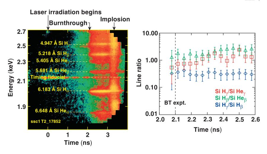
$\bullet$  Burnthrough T<sub>e</sub> ~ 750 eV is inferred from measured line ratios.
