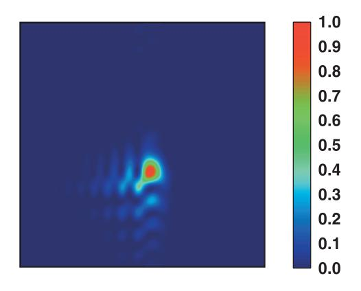
• The image spot size at the 10% level is less than 15  $\mu$ m (box size is 30  $\mu$ m). A division by the magnification M = 6 yields 2.5  $\mu$ m resolution in the object plane.
