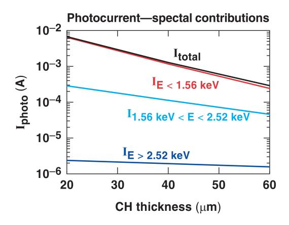
• Spectral partitioning of the PJx current shows no contrast impairment due to hard-x-ray-induced photocurrent.
