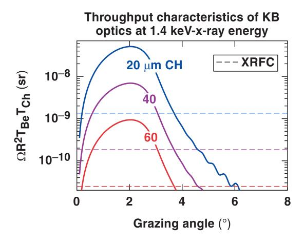
Comparison of the microscope with a gated pinhole array (XRFC) shows a solid angle improvement of two orders of magnitude at the optimal angle of incidence.
