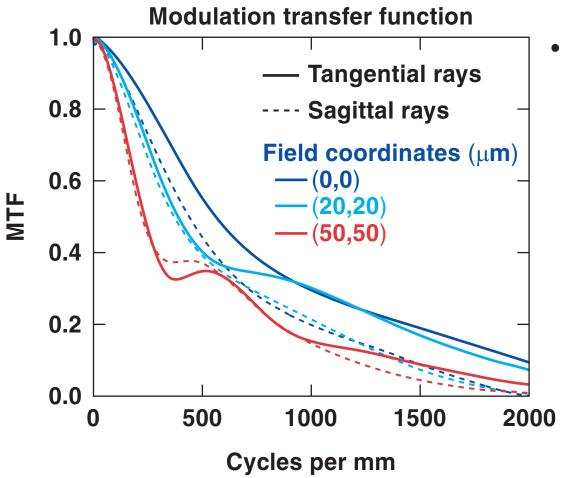
For 5-μm wavelength (200 cycles per mm) the MTF is greater than 0.6 at all three fields and for both tangential\* and sagittal rays.
