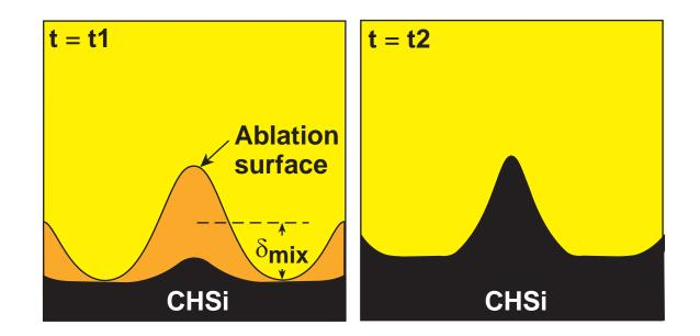
The time for CHSi to reach the tip of the spike is calculated by assuming that the rate of removal of the CH in the spike is given by the 1-D mass-ablation rate.
