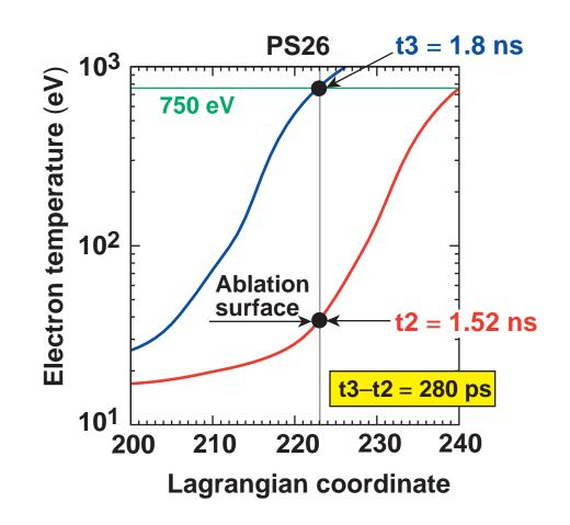
$T_e$  profiles at times when a fluid element is at the ablation surface (t2) and when it reaches the 750-eV isotherm (t3) .
