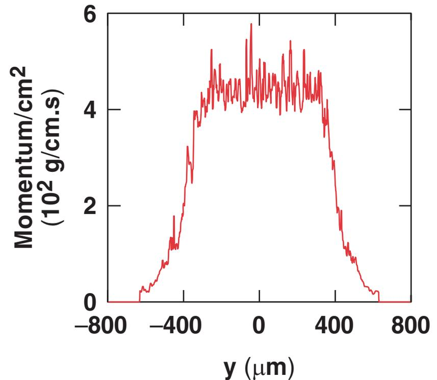
At 1 ns, the target momentum shows comparable modulation amplitudes but less short-wavelength structure
