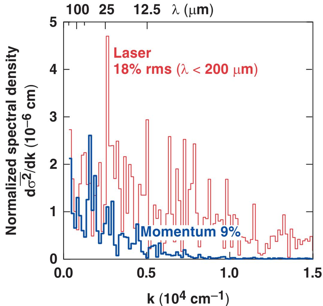
At 1 ns, the imprint is dominated by 20- to 50- $\mu\text{m}$  wavelengths
