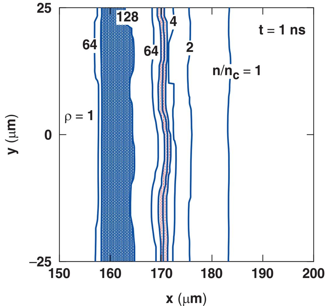
The heat deposition region is narrow at early times and close to the ablation front (A)
