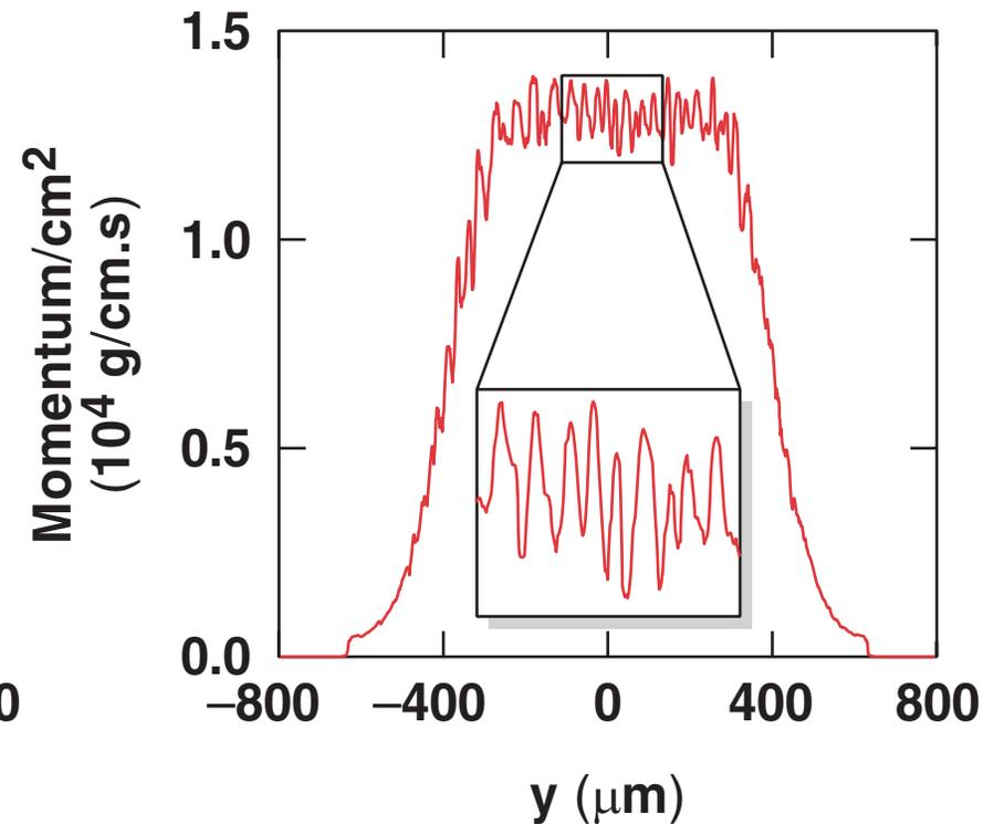
At 100 ps the target response shows less  $\sigma_{\text{rms}}$ , especially for shorter-wavelength modes
