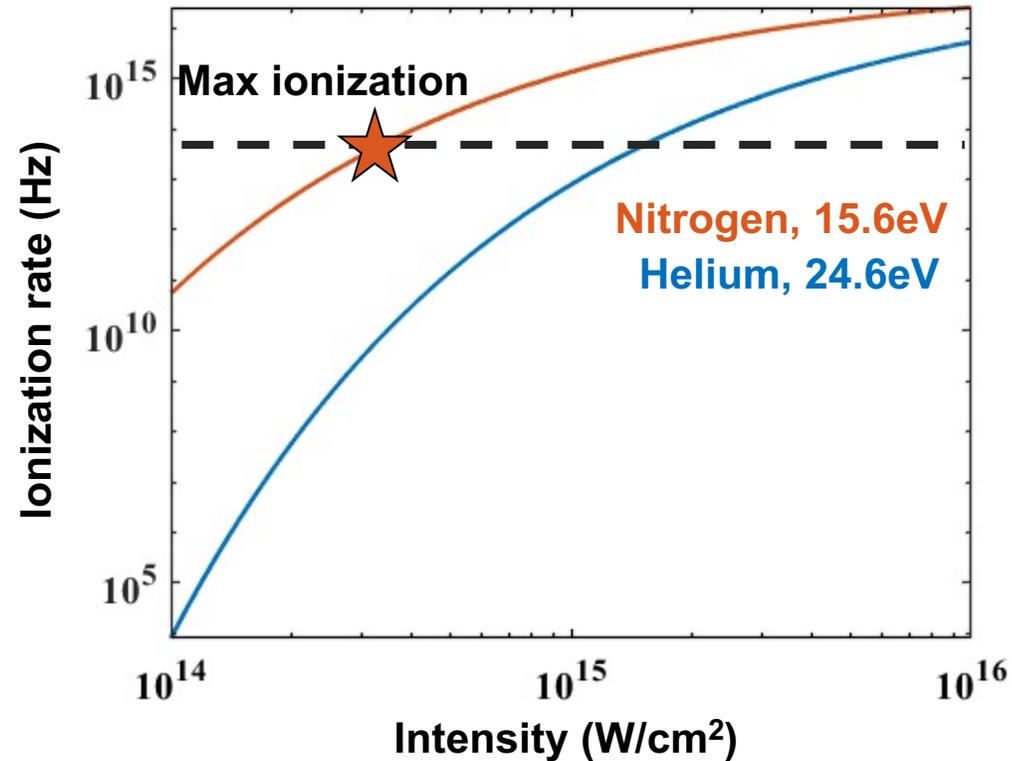
For a 15fs drive pulse in  $10^{17}/\text{cc}$  density gas,
