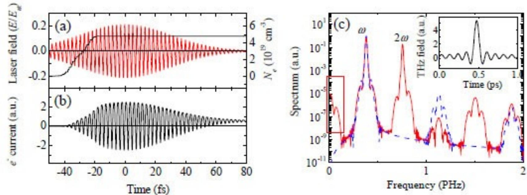
The combination of ionization and the net drift velocity induced by the asymmetric two-color field generates THz radiation
