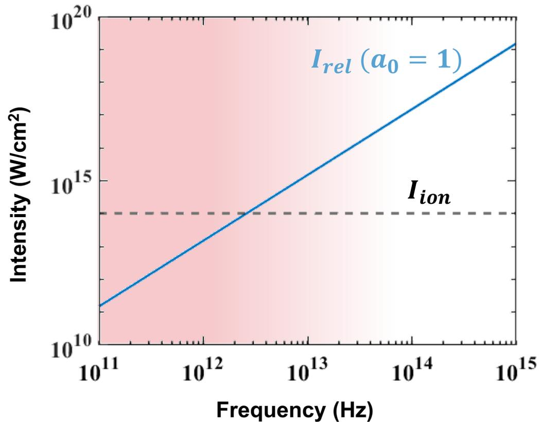
A high-energy terahertz source could enable access to a 'wavelength frontier' where bound electron nonlinear optics and relativistic plasma physics overlap
