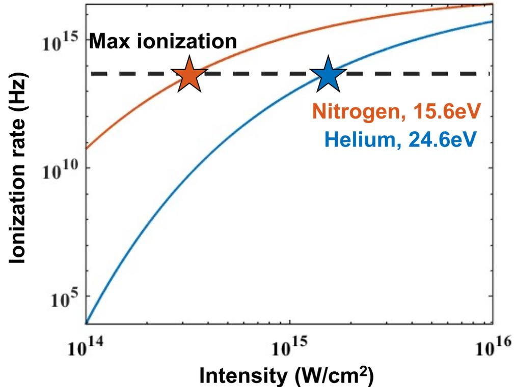
For a 15fs drive pulse in 10<sup>17</sup>/cc density gas,
