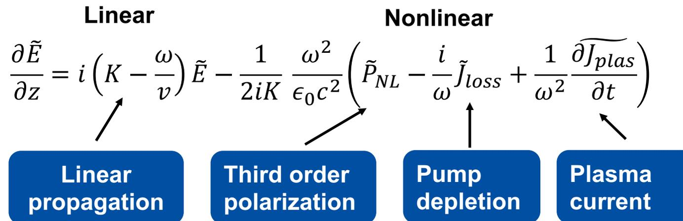
The terahertz is primarily produced via the transient plasma current
