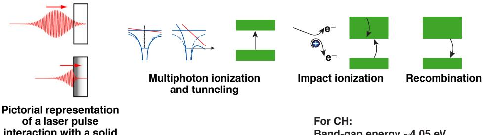
Band-gap energy ~4.05 eV UV light,  $\lambda$  = 351 nm, E = 3.53 eV Critical density: 9 × 10<sup>21</sup> cm<sup>-3</sup>
