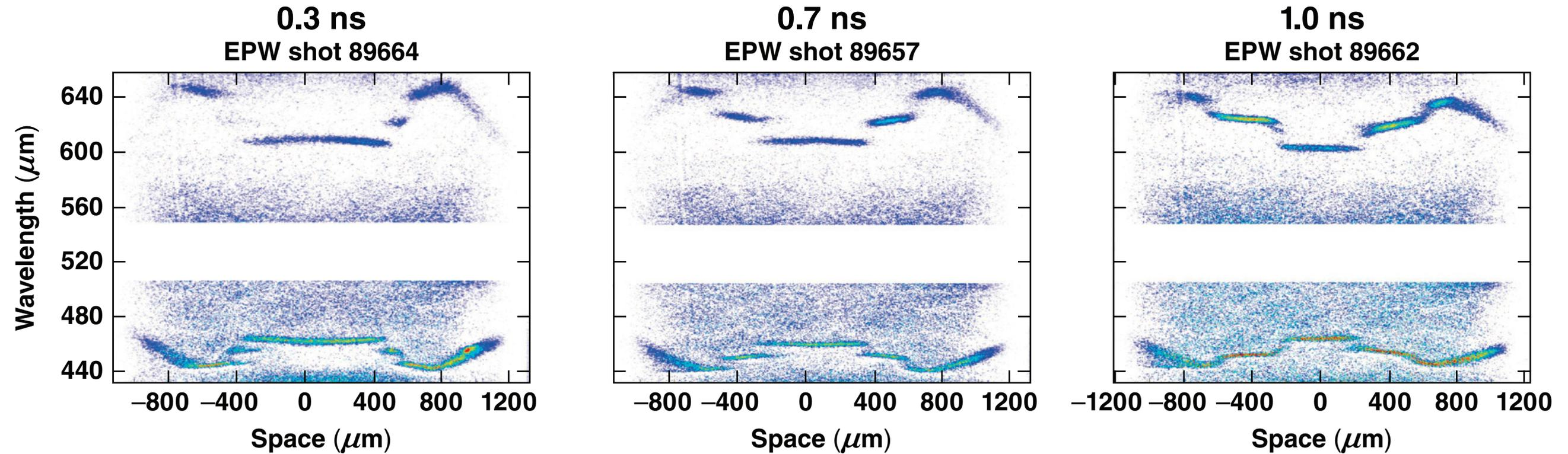
Density perturbations are caused by neutral density flow properties in the supersonic nozzle.
