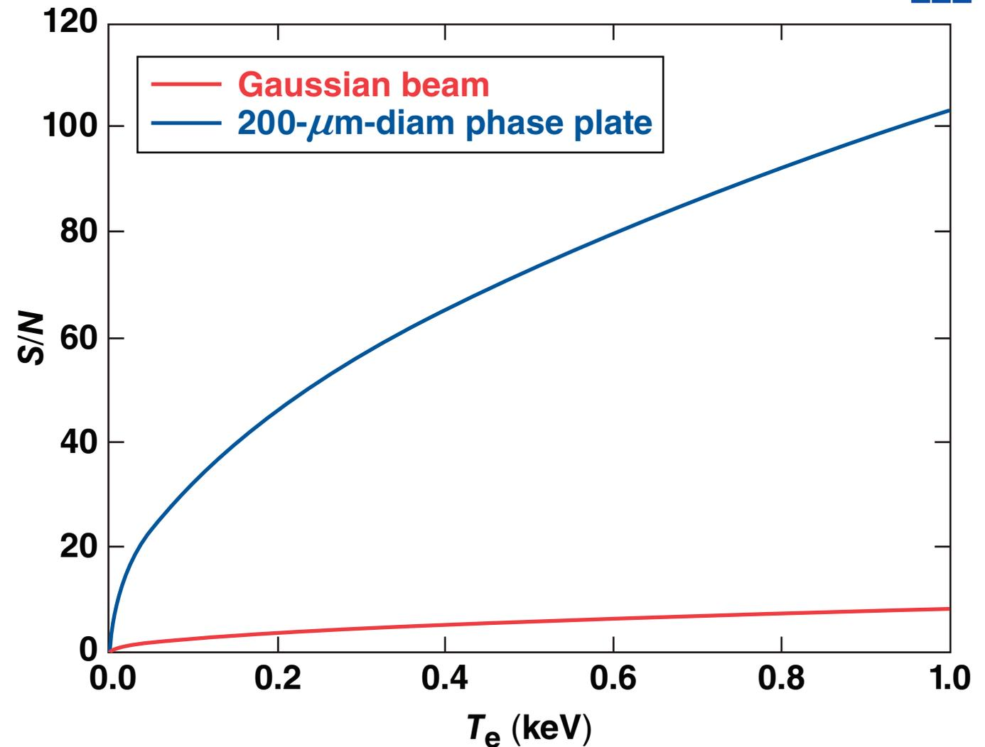
A 200-μm-diam phase plate was used to improve propagation.
