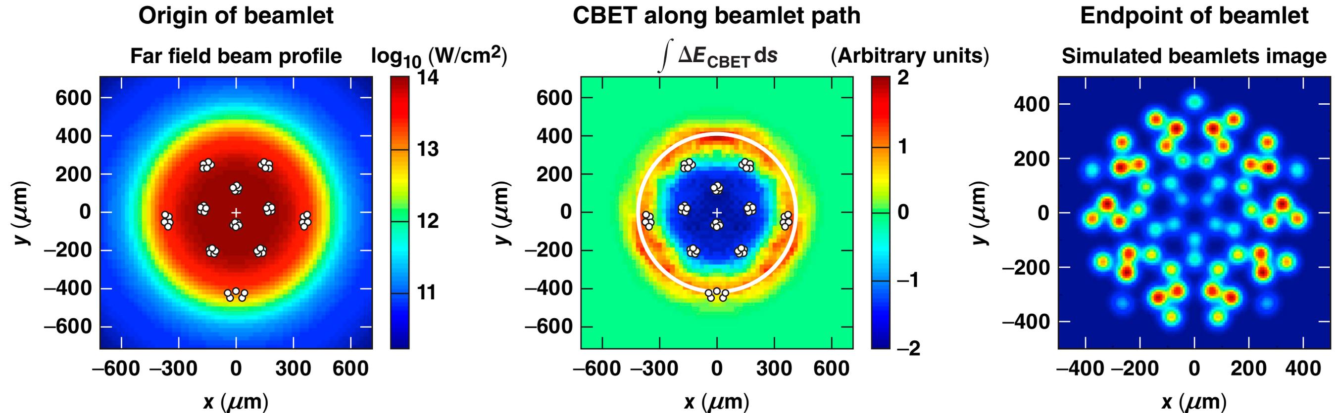
Each spot is the endpoint of a beamlet originating from a specific location of the beam profile and experiencing CBET differently because their unique paths
