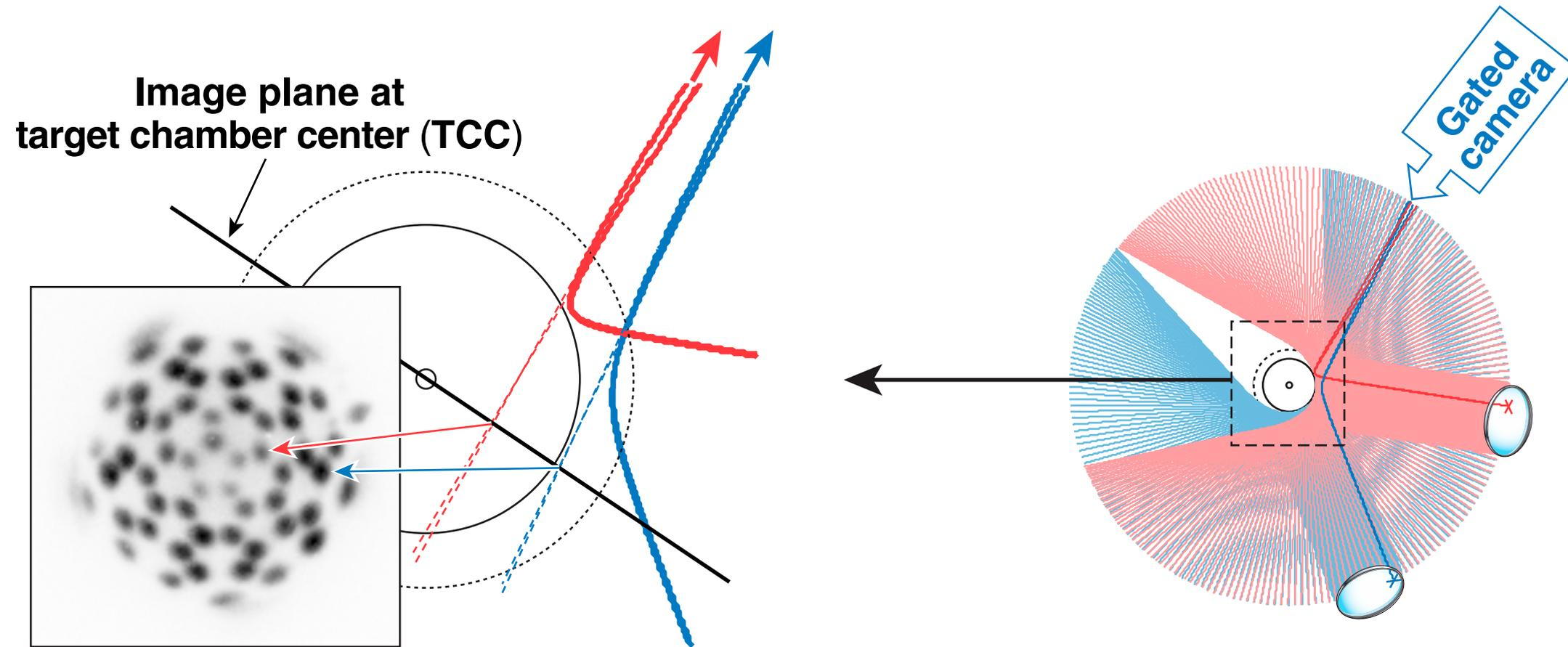
Each spot is the endpoint of a beamlet originating from a specific location of the beam profile and experiencing CBET differently because their unique paths
