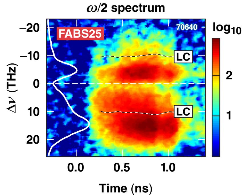
NIF SRS spectra are observed at 23°, 31°, and 50° and identify SRS sidescattering is the dominant process
