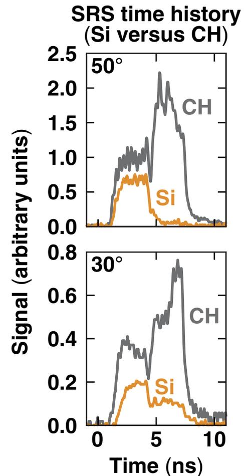
In comparison to the CH target, the Si target produced an  $\sim 30\%$  lower  $f_{\text{hot}}$  and an  $\sim 15$  keV lower  $T_{\text{hot}}$  for small-angle-beam drive
