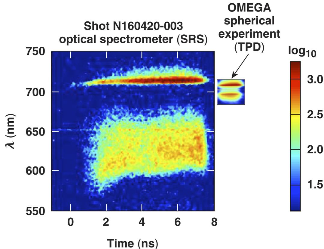
On the NIF, the observed  $\omega/2$  emission is attributed to absolute SRS, although the presence of TPD cannot yet be ruled out.
