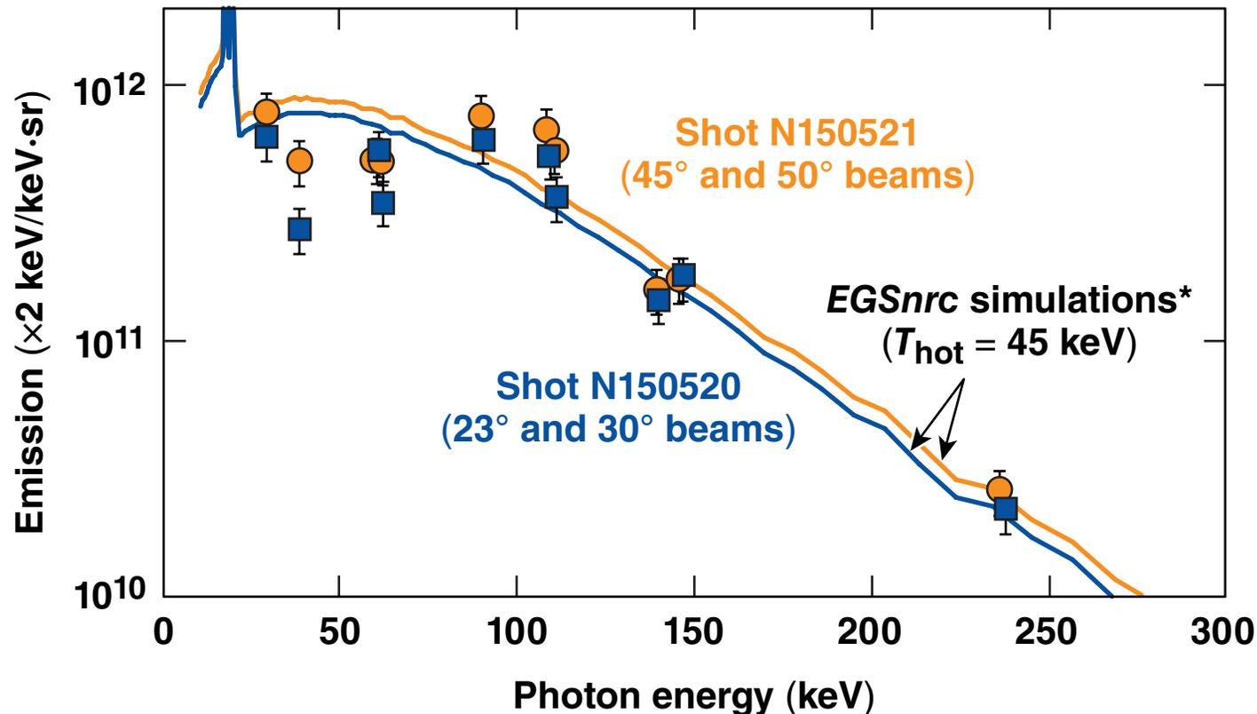
The beam angle of incidence did not have a strong effect on  $f_{\text{hot}}$  and  $T_{\text{hot}}$ .
