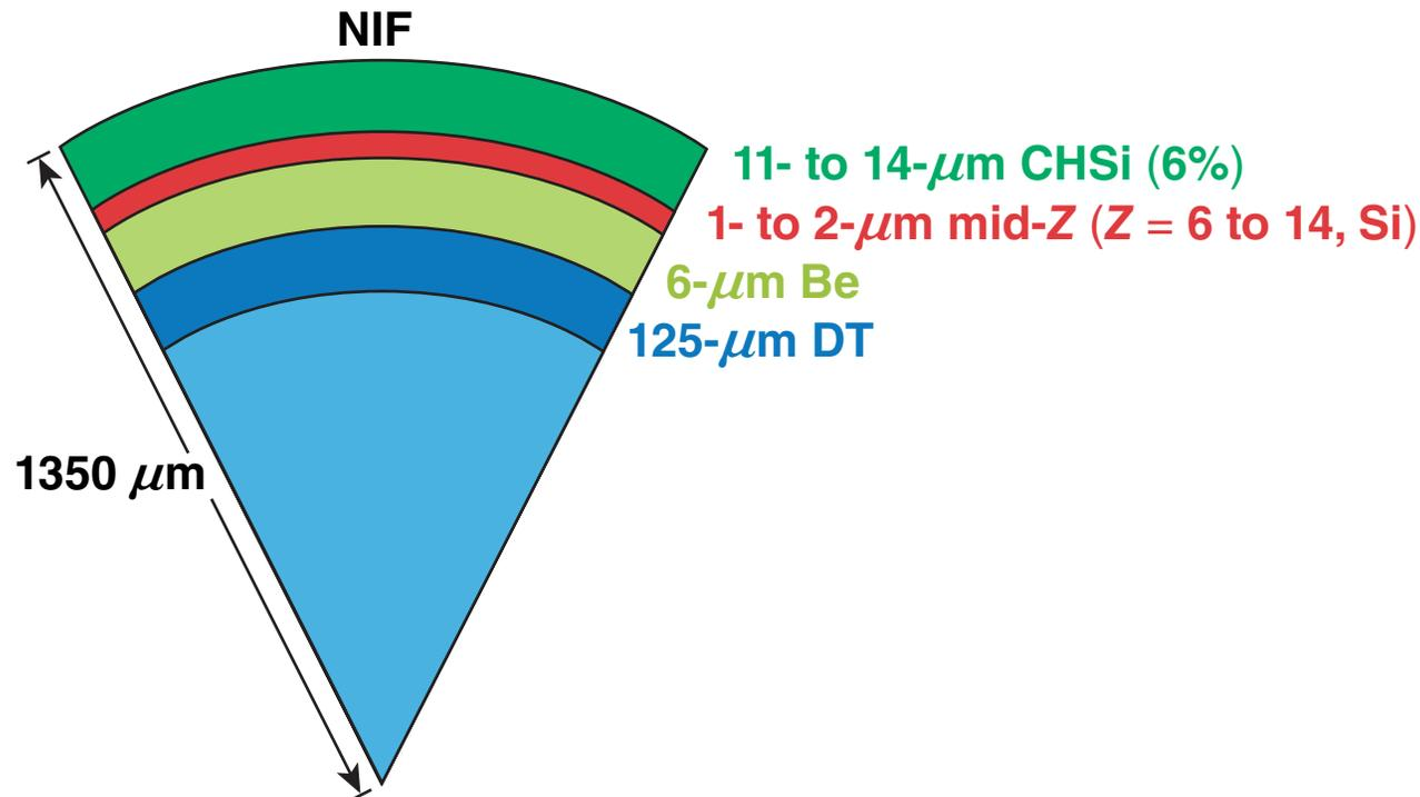
Si ablators produce shorter scale lengths, higher electron temperatures, and more collisional damping in order to reduce LPI near  $n_c/4$ .
