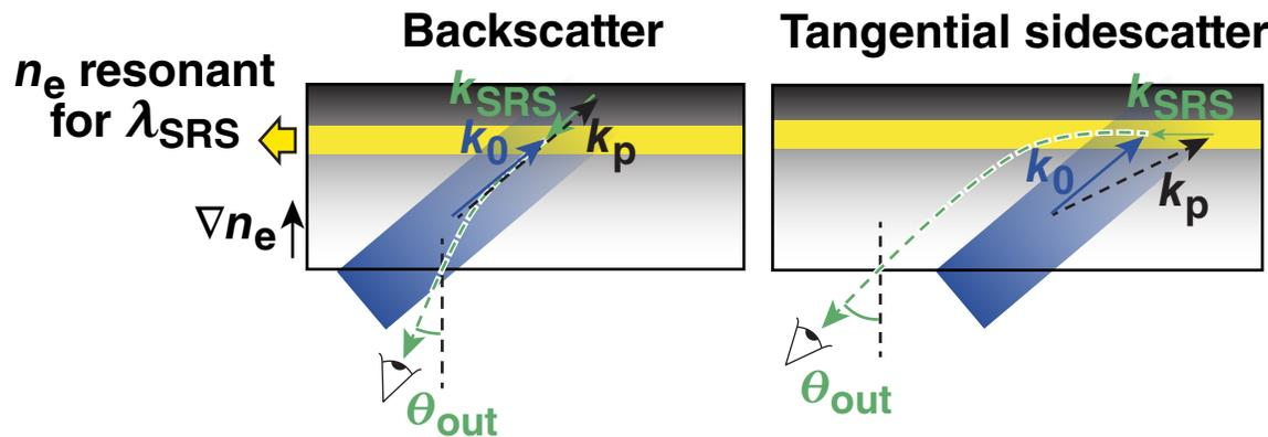
Tangential sidescatter exit angle does not depend on the incidence angle
