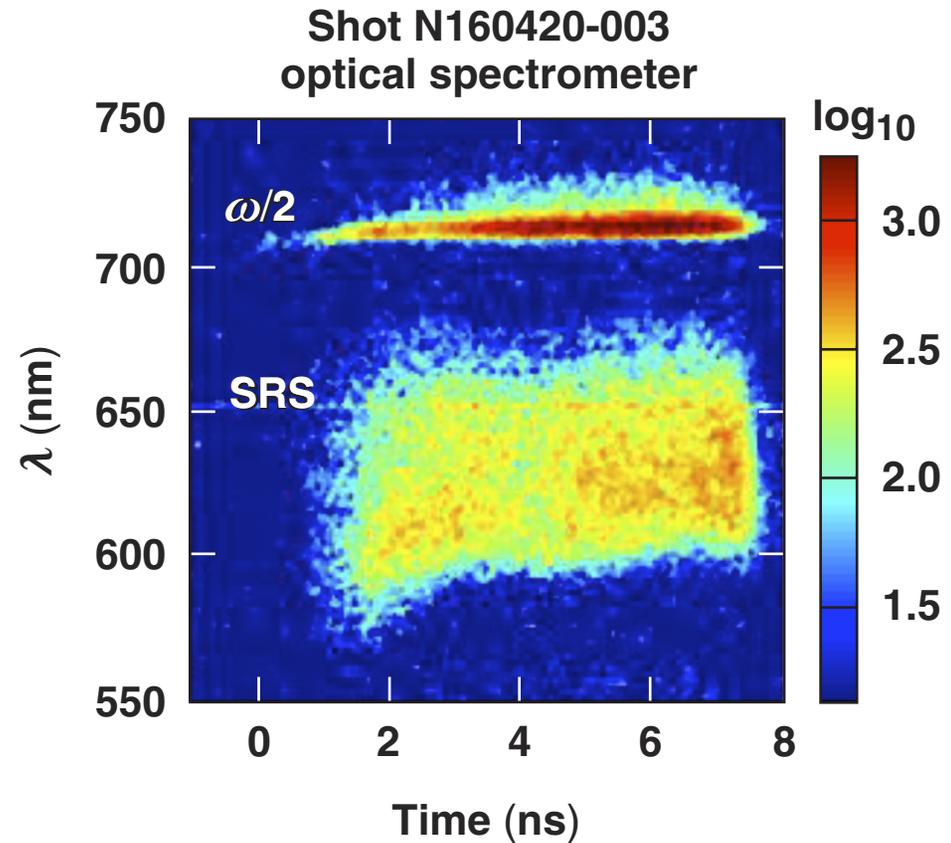
The  $\omega/2$  feature observed on the NIF is in contrast to that observed on OMEGA, which showed both blue- and red-shifted  $\omega/2$ , and is attributed to TPD
