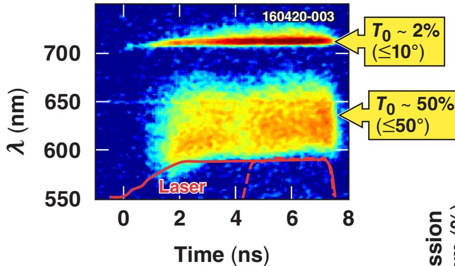
Distribution of observed sidescattered SRS based on ray-tracing of 2-D simulated plasma conditions
