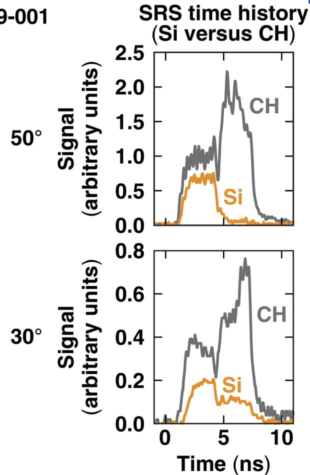
For an Si ablator, the SRS intensity at 23° depends strongly on inner-beam laser intensity, but SRS observed at 50° is still minimal
