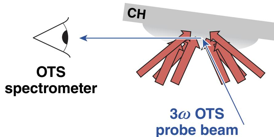
These experiments will assess the presence of TPD, confirm plasma conditions, and develop a platform for eventual use of  $5\omega$  Thomson scattering (TS) to probe plasma waves.
