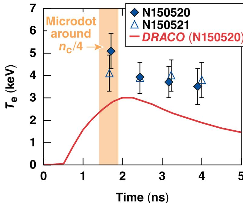
Based on modeling, discrepancy can be partially explained by self-heating of the microdot.
