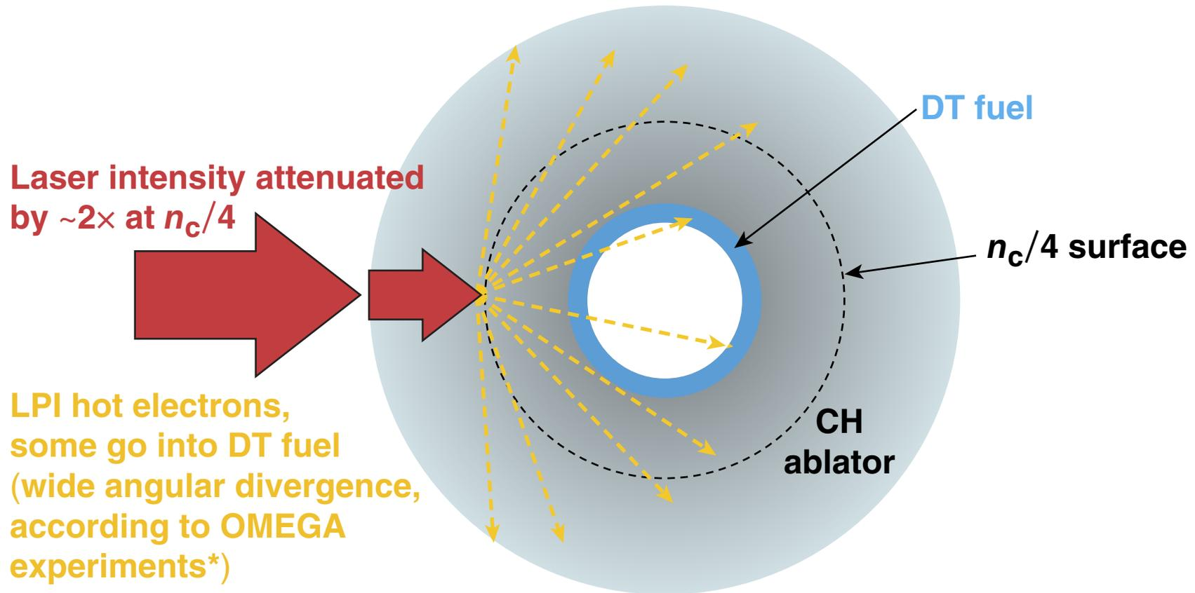
**Limit of  $\sim 0.15\%$  laser energy into fuel preheat + angular divergence
