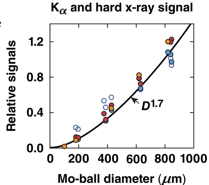
The increasing  $K_{\alpha}$  signal with Mo shell diameter on OMEGA indicated a wide angular divergence in the TPD regime.
