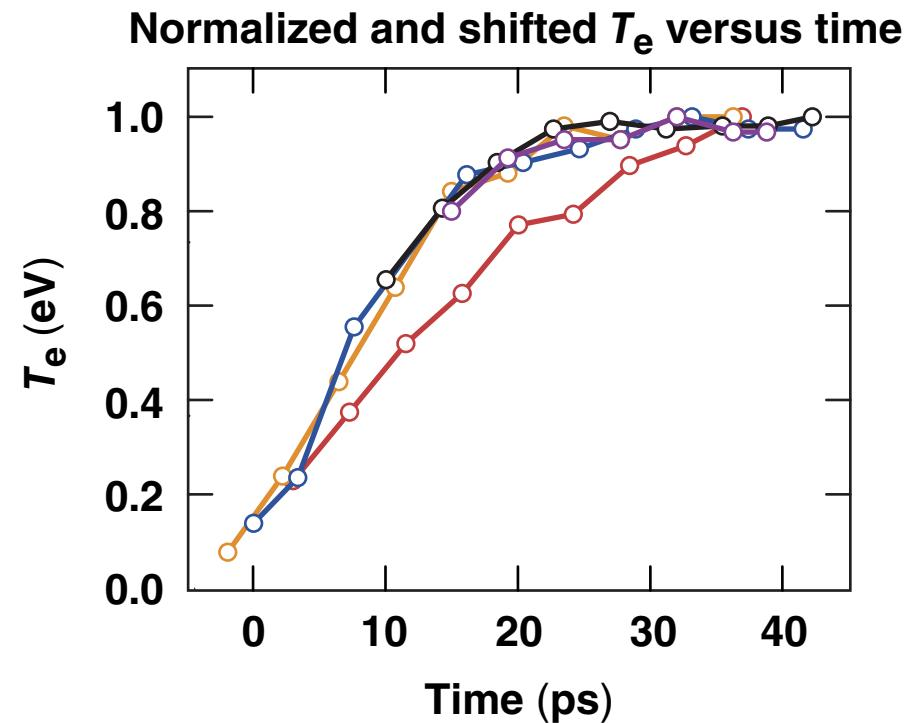
The electron temperature was observed to rise from an initial 5 eV to a density-dependent plateau in 23 ps.
