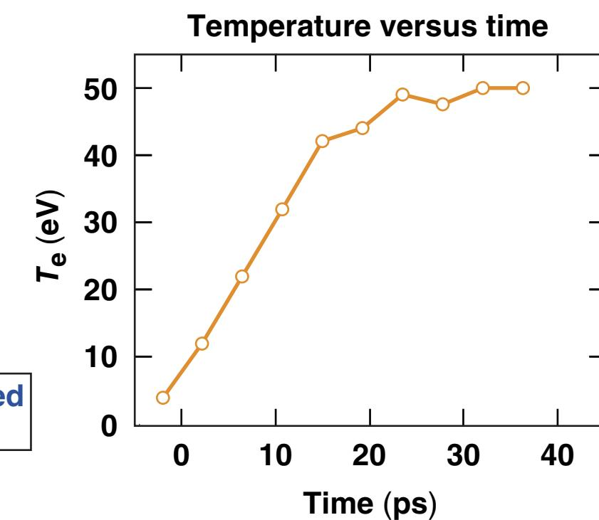
The heating rates and temperature plateaus were measured as a function of density for a  $2 \times 10^{14} \text{ W/cm}^2$  pump laser
