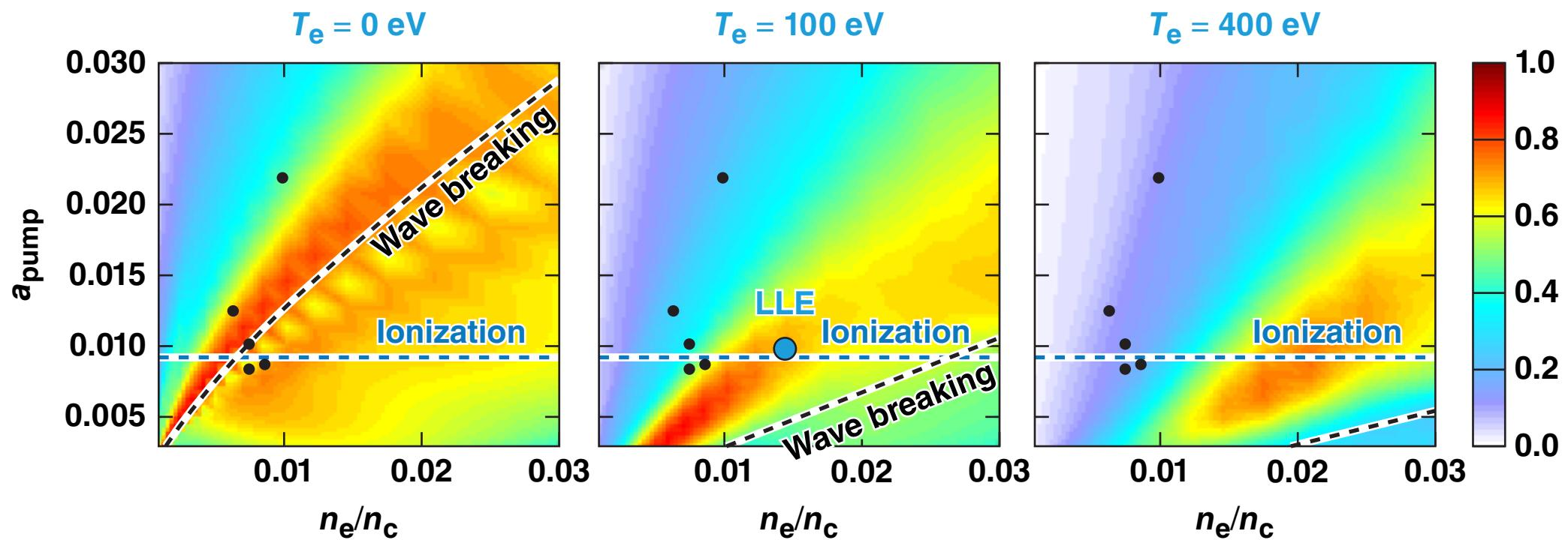
Wave breaking changes the parameter regime for optimal efficiency in a Raman amplifier.
