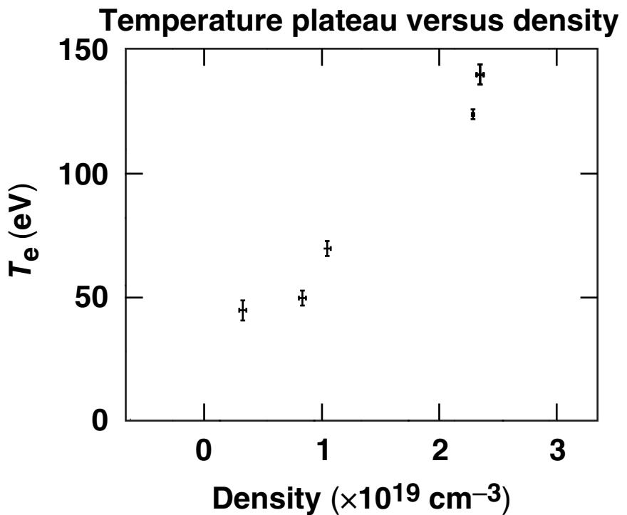
The electron heating rate and plateau temperature are found to increase with higher densities.
