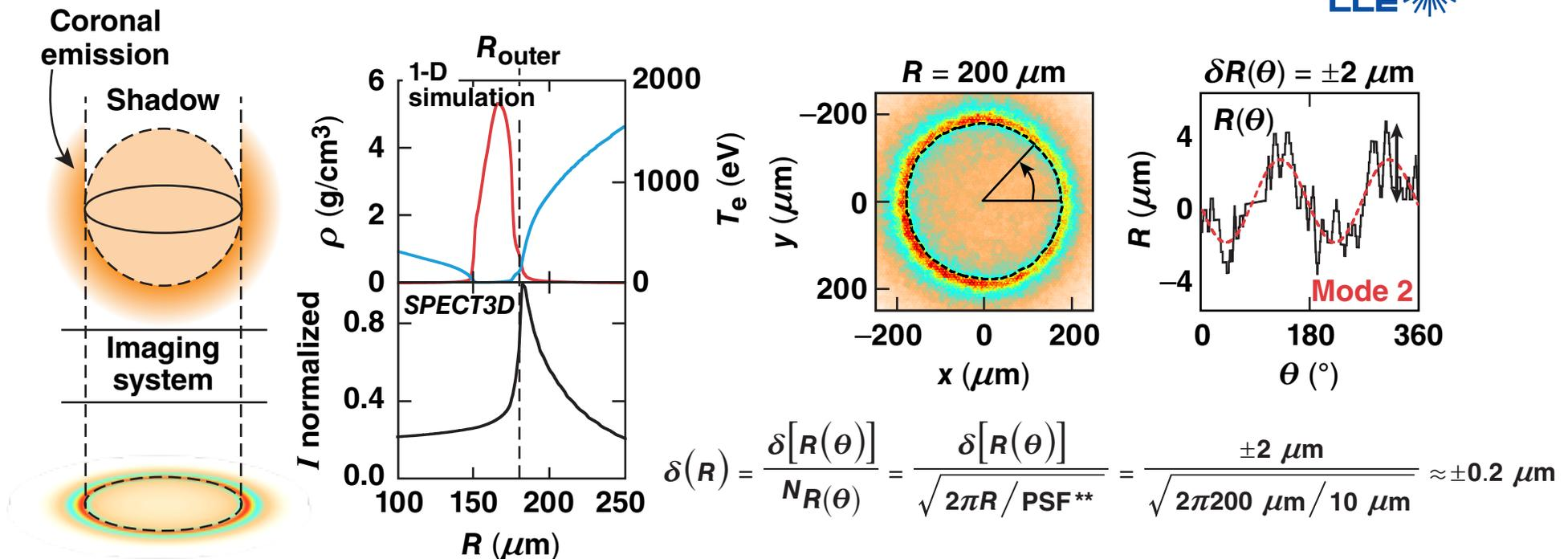
The shadow effect prevents the emission coming from the back of the shell from reaching the diagnostic, reducing the emission by a factor of 2 just after the outer edge of the shell.
