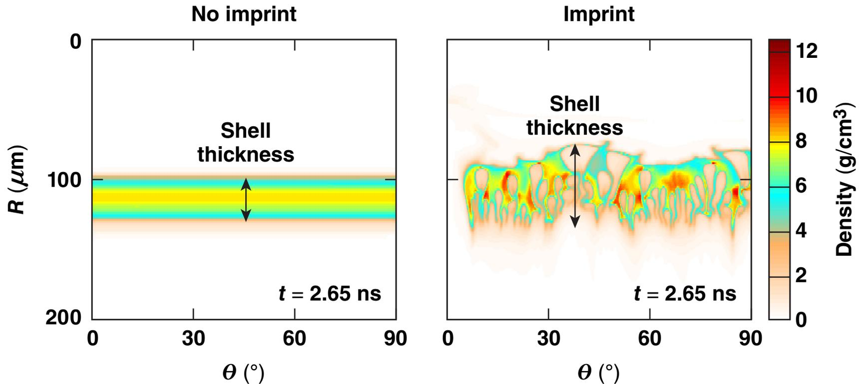
The decompression of the shell reduces the shell pressure and the implosion performances.
