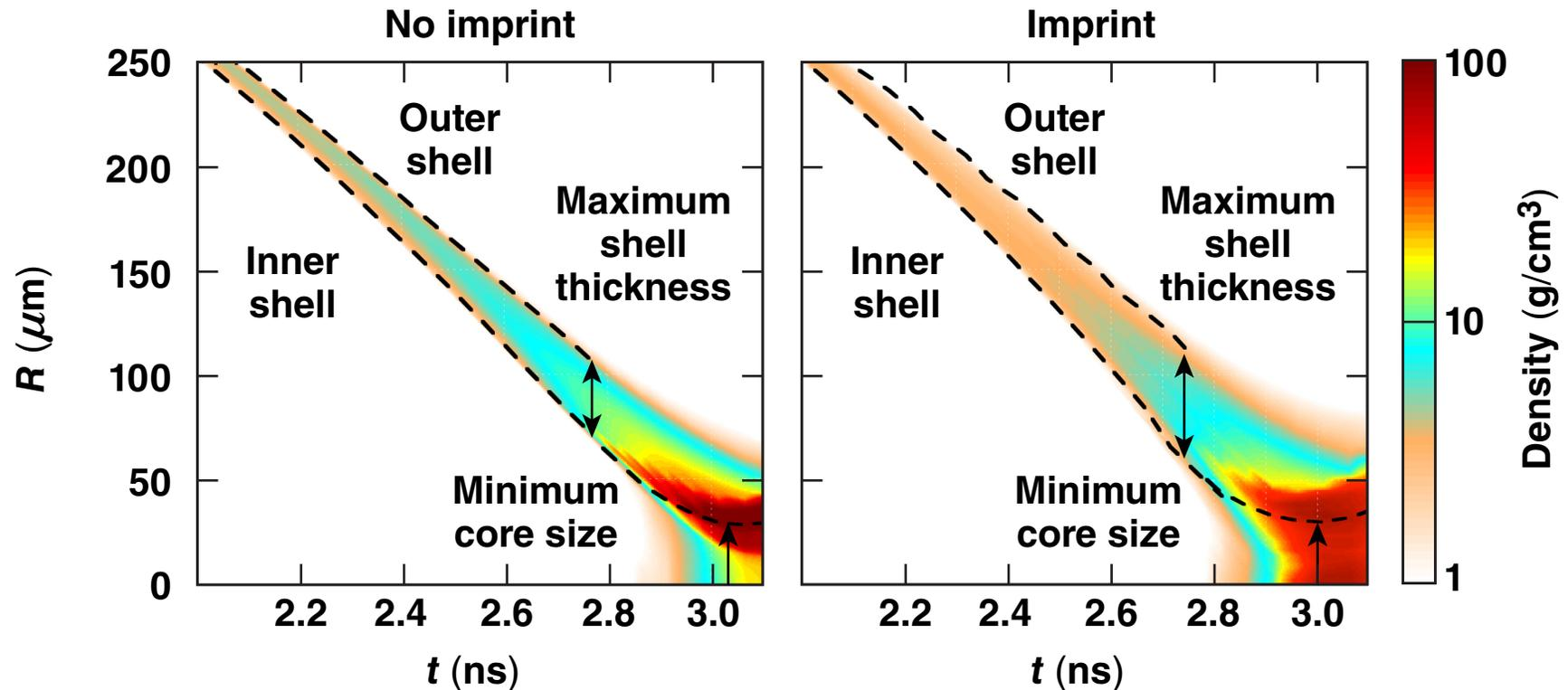
**Nonuniformities increase the thickness of the shell but not the minimum core size.**
