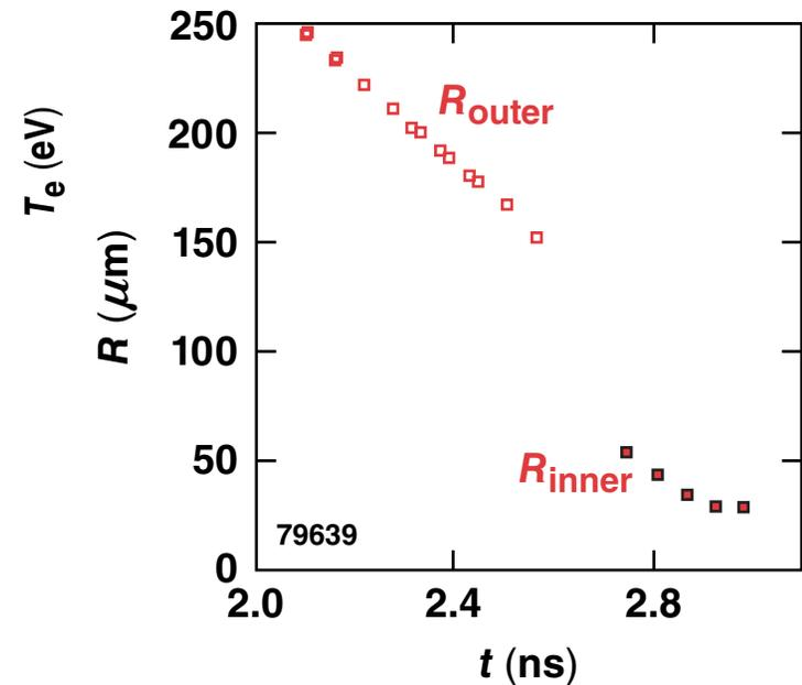
The outer and inner surfaces of the shell are measured from self-emission images within  $\pm 0.2 \mu\text{m}$  and  $\pm 2.0 \mu\text{m}$ , respectively
