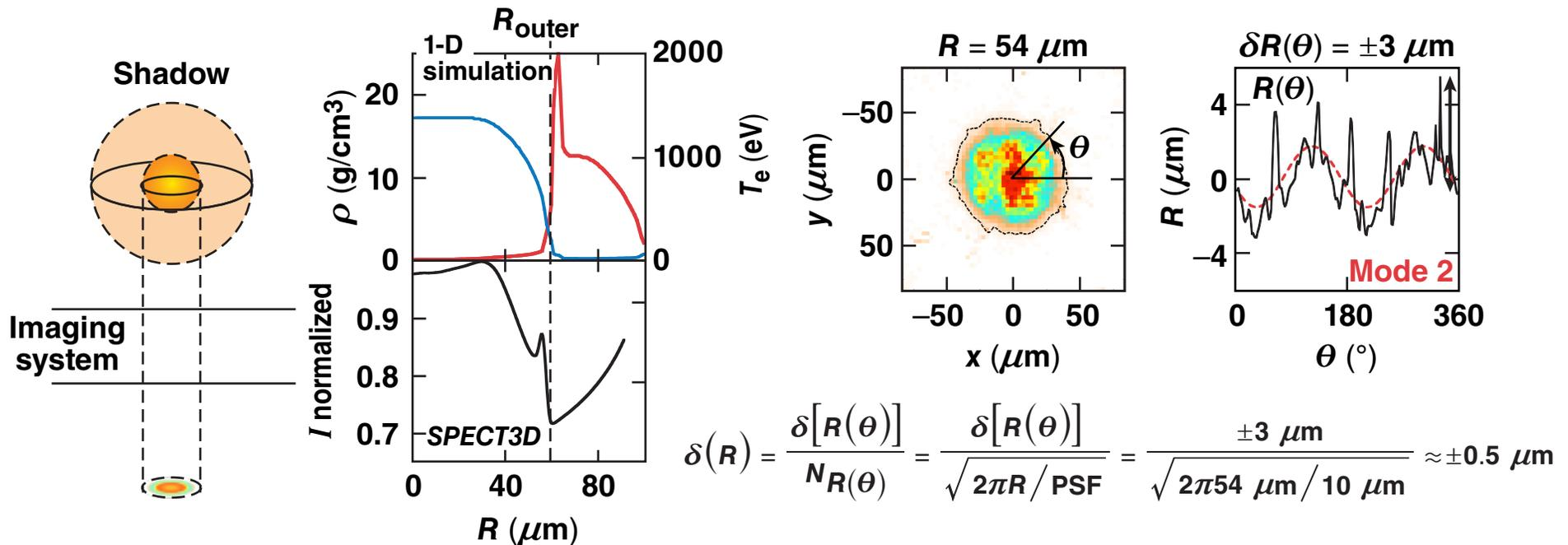
The outer surface of the core emission makes it possible to determine the inner surface of the cold shell within  $\pm 0.5 \mu\text{m}$ .
