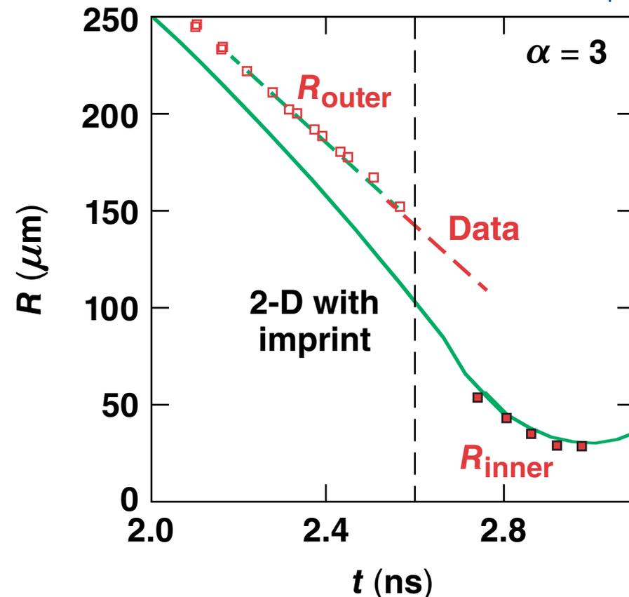
The simulation reproduced the shell thickness and deceleration.
