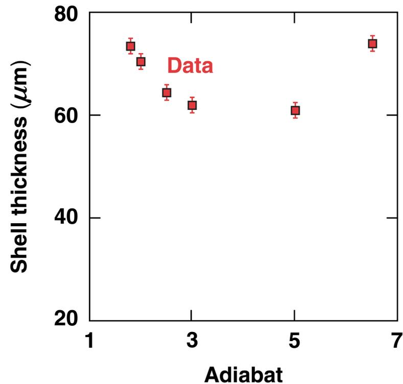
This shows that the shell decompression observed for a low adiabat is not caused by an error in the adiabat calculation.
