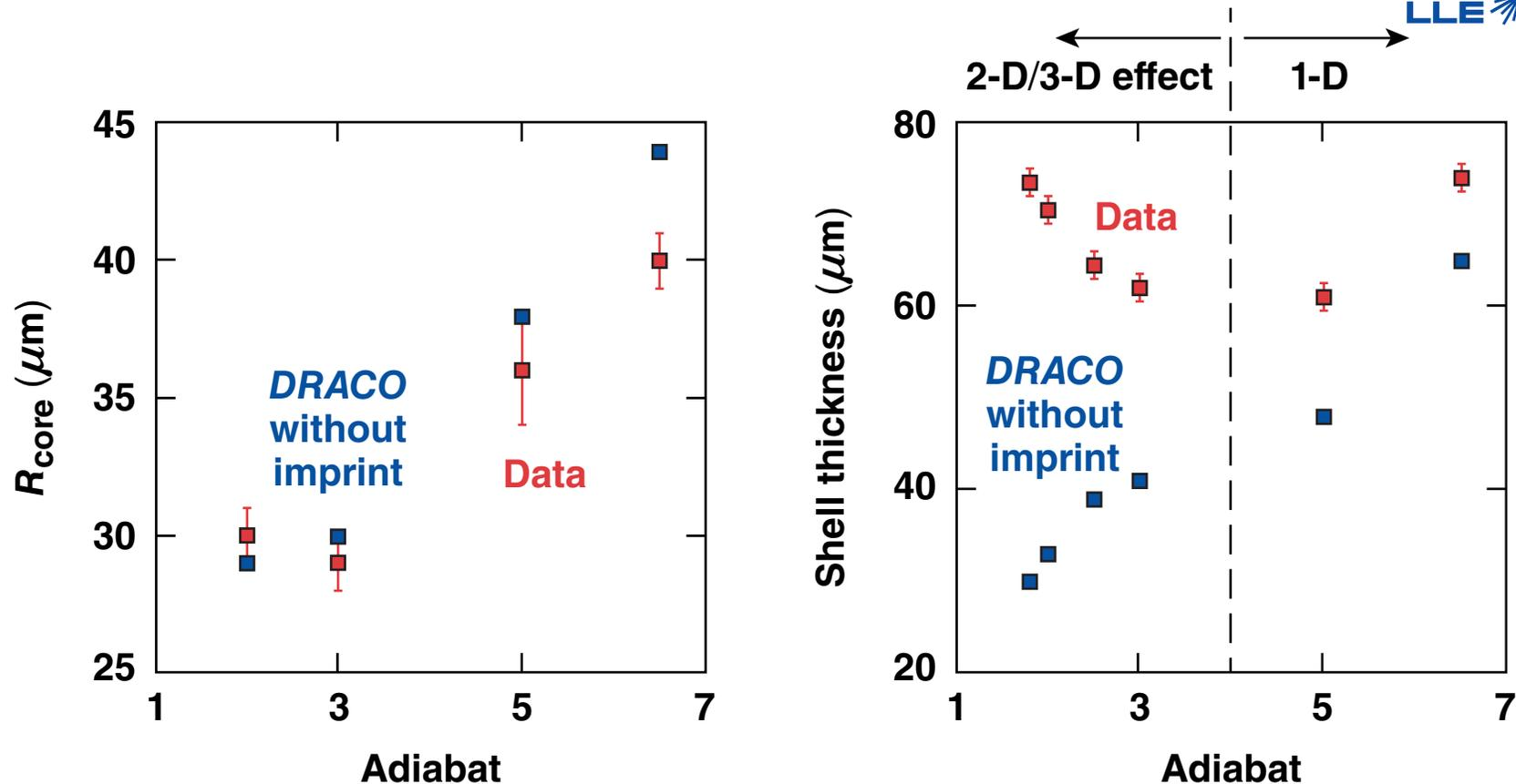
For a lower adiabat ( $\alpha < 4$ ), significant shell decompressions are observed because of 2-D/3-D effects.
