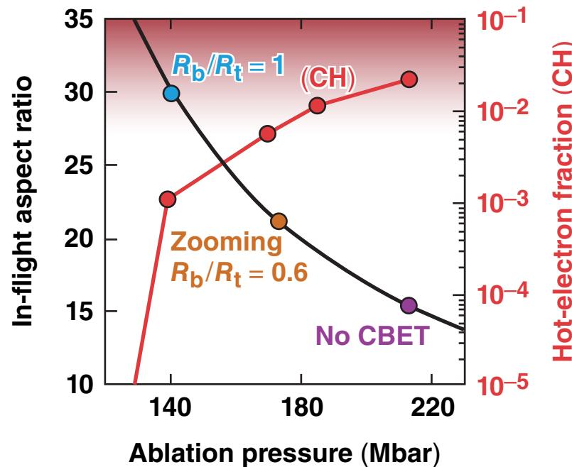
Current cryo experiments show no evidence of hot-electron preheat, but simulations suggest a factor-of-2 increase will degrade the areal density.
