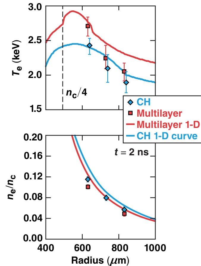
Multilayer ablators increase the electron temperature around quarter critical by ~15%.
