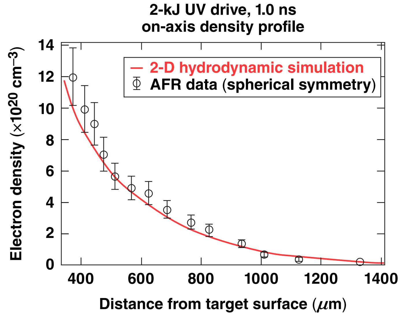
The plasma scale length is measured to be  $250 \mu\text{m}$  by AFR.
