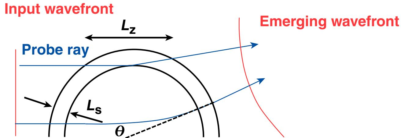
Phase shift through plasma  $\Phi = \frac{\omega}{c} \int_0^{L_z} N dl = \frac{\omega}{c} \int_0^{L_z} \sqrt{1 - \frac{n_e}{n_c}} dl \approx \frac{\omega}{2cn_c} \int_0^{L_z} n_e dl$
