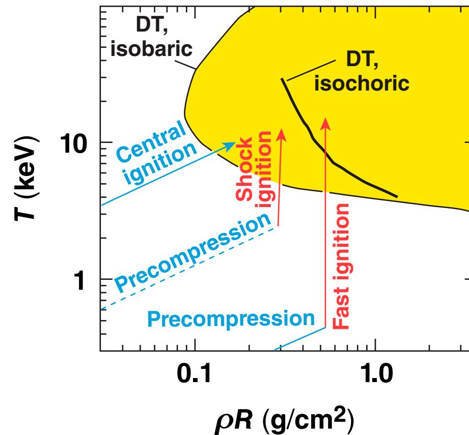
For electron FI, the goal is to get the source close to the compressed core.
