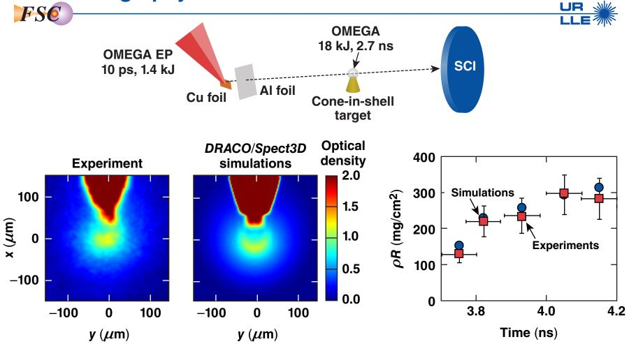
Cone-tip breakout time agrees in the experiments and simulations but is ~200 to 300 ps before the peak compression time
