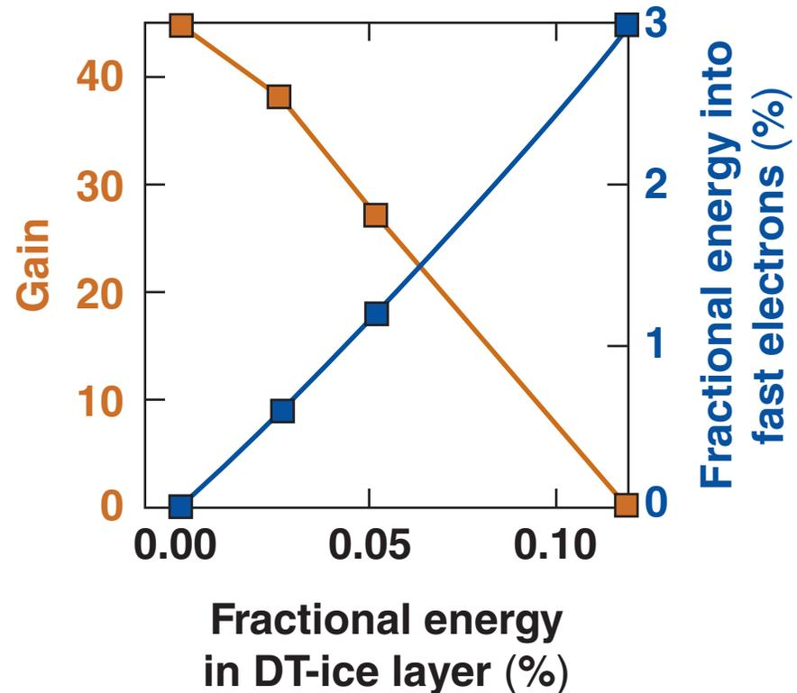
Calculations suggest that the fraction of laser energy converted to hot electrons should be kept low\*.
