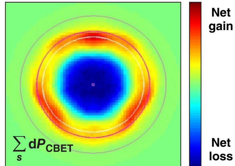
Power transferred in/out of beamlets is integrated along the path of each beamlet
