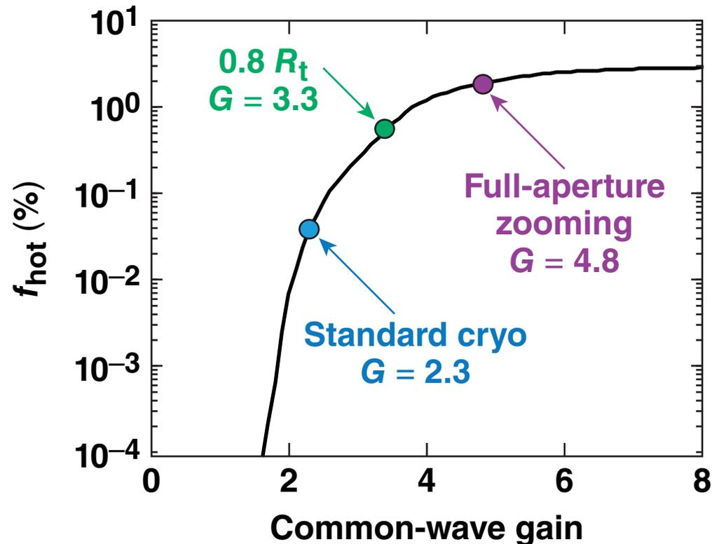
If CBET mitigation is needed to get a stable hydro-equivalent implosion, the TPD gain and hot-electron production will increase.
