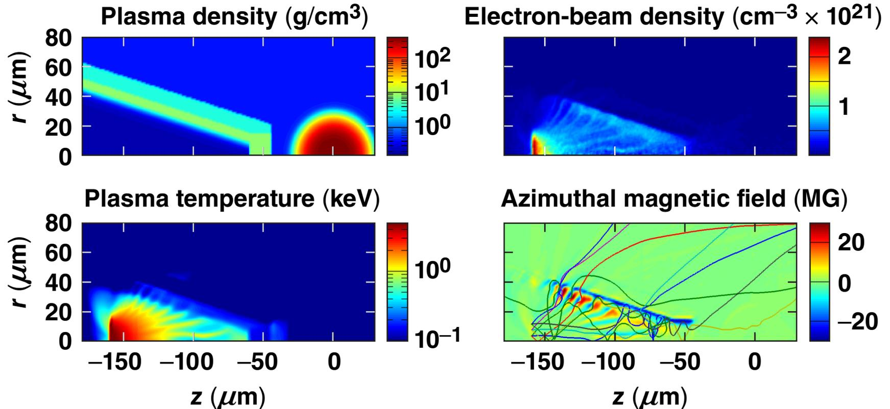
**Electrons collimated to the cone tip contain 17% of the beam energy.**
