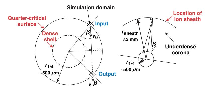
The delay at the inner boundary is short, with significant energy loss; the delay at the outer boundary is long, with little energy loss
