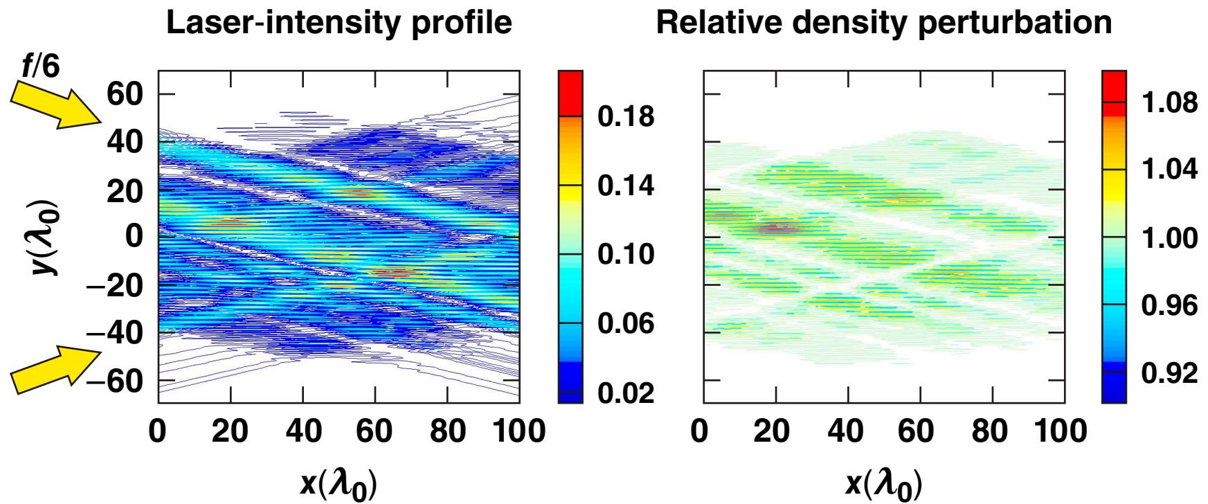
$$\langle I \rangle = 9 \times 10^{14} \text{ W/cm}^2, \quad T_e = 2 \text{ keV}, \quad n_0 \approx \frac{n_c}{4}, \text{ CH} \quad \left( \frac{n_e}{n_0} - 1 \right) \sim \frac{I}{\langle I \rangle}$$
