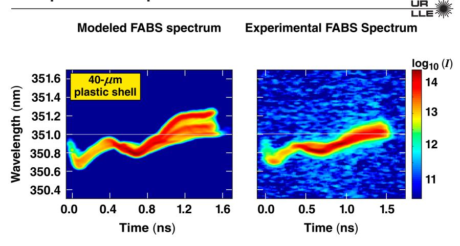
Reduced absorption is likely concentrated in the beams best coupled to target ablation surface.
