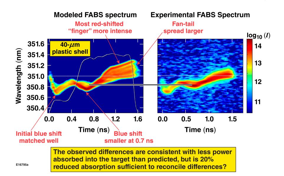
Modeling with a pulse scaled to give the experimentally observed absorption does not significantly improve the spectral shift predictions
