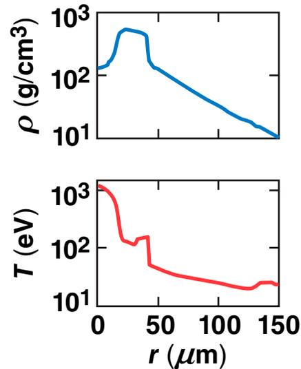
Gaussian (in  $r$ ) e-beam with FWHM =  $30\ \mu\text{m}$  and duration  $\tau = 5\text{ps}$ ,  $\langle E_e \rangle = 2.2\ \text{MeV}$ ,  $\Delta E_{\text{th}} = 0.3 \langle E_e \rangle$ , opening half angle =  $20^\circ$
