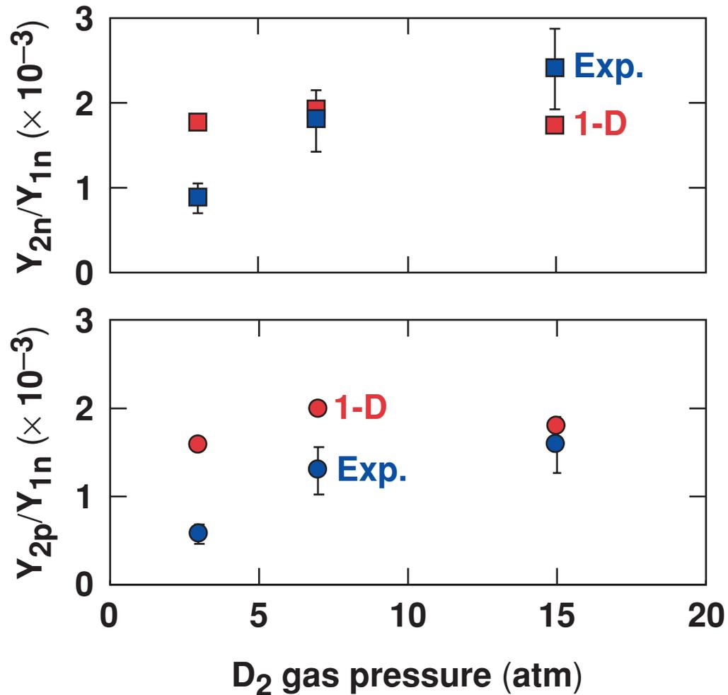
Experiments with a 1-ns square laser pulse show no truncation of burn for 15-atm implosions, but ~20% truncation of burn for 3-atm implosions
