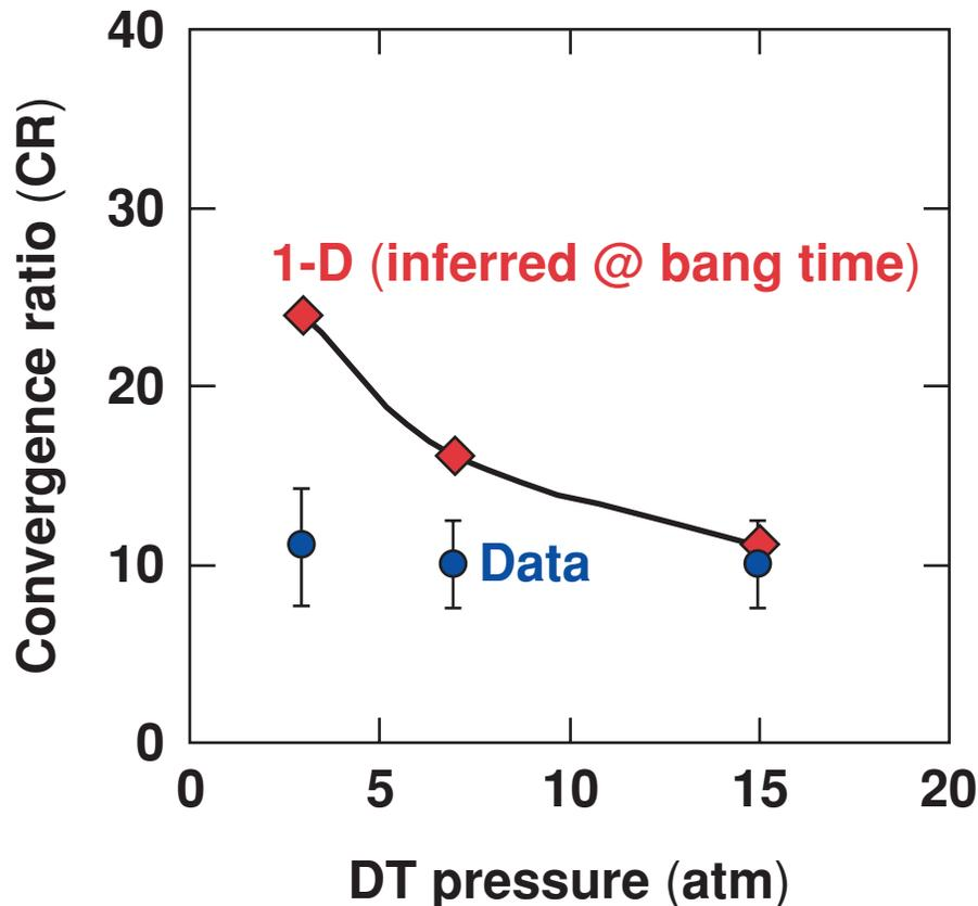
CR is determined by either  $\rho R_{\text{fuel}}$  or  $\rho R_{\text{shell}}$  measurements:
