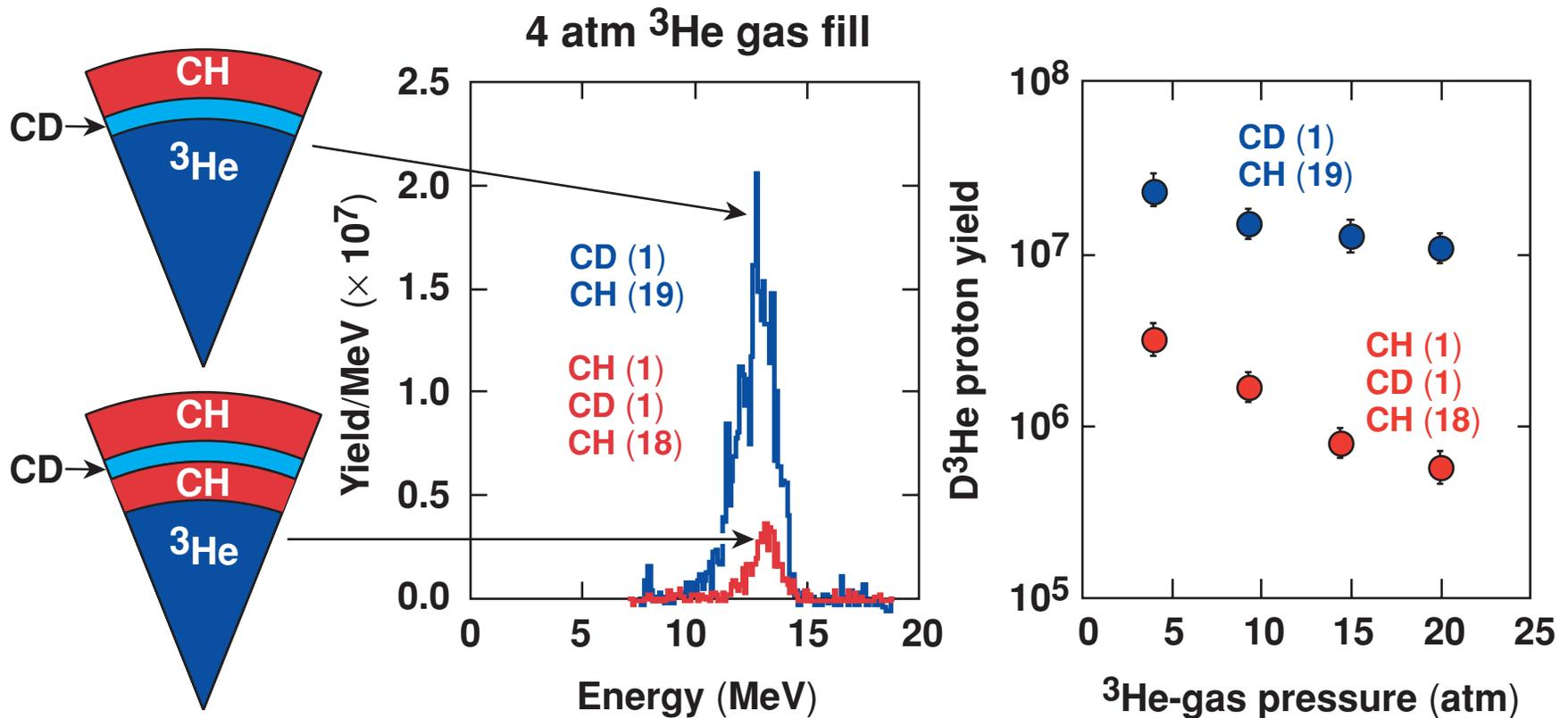
Implosions of 15-atm capsules achieve ~85% of 1-D predictions for both  $\rho R_{\text{fuel}}$  and  $\rho R_{\text{shell}}$ , while 3-atm capsules achieve ~25% for  $\rho R_{\text{fuel}}$  and ~60% for  $\rho R_{\text{shell}}$
