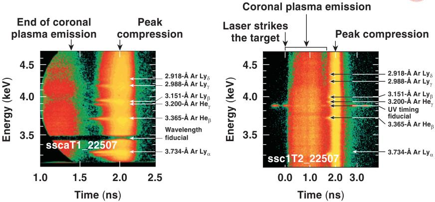
Absolute timing of peak x-ray signal is established with a slower streak camera.
