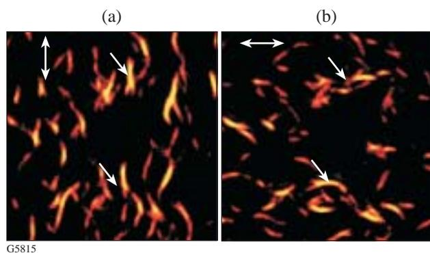
Figure 93.55 Confocal Raman images of SWNT bundles produced by arc discharge on glass acquired by detecting the intensity of the *G'* band ( $\nu = 2615 \text{ cm}^{-1}$ ) while raster-scanning the sample (without metal tip, scan area  $15 \times 15 \mu\text{m}$ ) for vertical (a) and horizontal polarization (b) of the laser excitation at 633 nm. The arrows indicate tubes that are oriented completely perpendicular to one polarization direction, demonstrating the polarization contrast.
