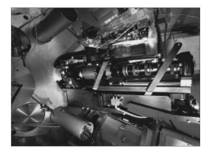
The Kowaluk camera is built around a commercially available 35-mm camera and lenses. A rigid mounting system was designed to allow accurate imaging of the 1-mm-diam target from outside the chamber wall. During the shot the illumination is provided by the 60 OMEGA 351-nm laser beams.
