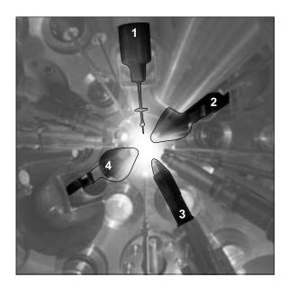
The photograph on the left defines the layout of the central cover photograph of the OMEGA target chamber by highlighting the key elements. The target positioner and the streaked x-ray crystal spectrograph are labeled 1 and 3, respectively, and the two time-integrated crystal spectrographs are labeled 2 and 4.
