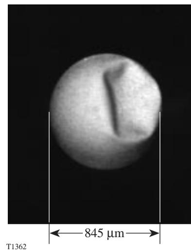
Figure 71.22 Plasma-assisted polyimide shell buckled at an external overpressure of ~36 atm. The shell did not brittle fracture, indicating a high fracture toughness.
