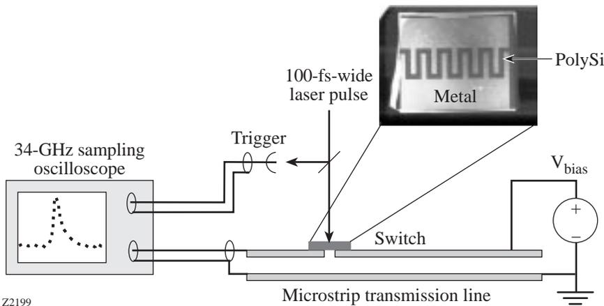
Figure 71.32 Sampling oscilloscope measurement setup. Inset shows the interdigitated switch geometry. Switch dimension is 2 mm × 2 mm; finger separation as well as finger width is 100 μm.
