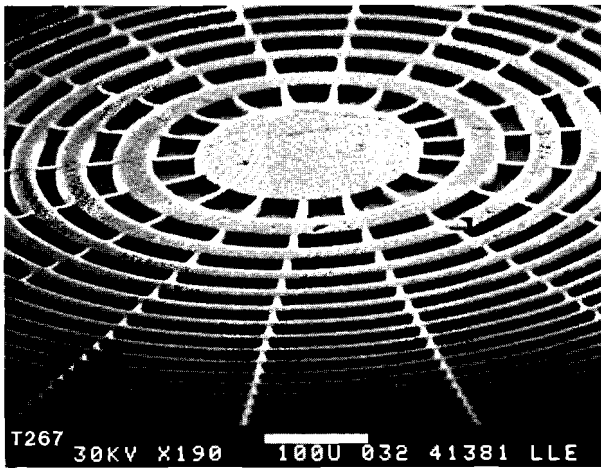
Fig. 28 A scanning electron micrograph of an intermediate RTV mold made from the Mylar master-pattern.
