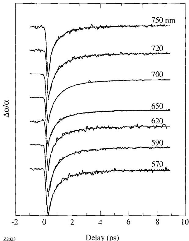
Figure 64.40 Time-resolved differential absorption ( $\Delta\alpha/\alpha$ ) of semiconducting YBCO at several probe wavelengths. The data are normalized and shifted vertically for clarity. The smooth lines are the fits using a stretched exponential.
