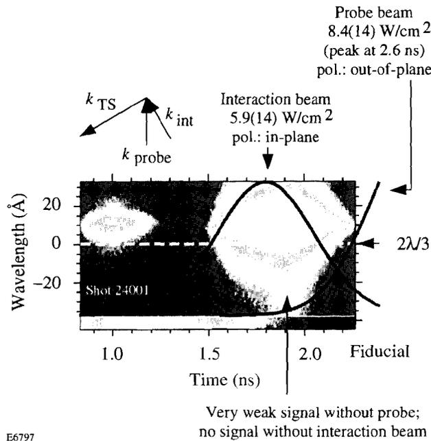
Figure 57.15 Direct evidence of TPD decay near the Landau cutoff using Thomson scattering. The TPD decay was driven by a particular secondary beam focused to  $\sim 6 \times 10^{14}$  W/cm<sup>2</sup> (averaged over the DPP speckle pattern). The Thomson probe beam was delayed to peak at 2.6 ns to avoid any accidental 3/2-harmonic generation from the probe beam itself.
