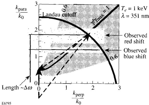
Figure 57.13 Two-plasmon decay diagram in  $k$ -space with  $k_{\parallel}$  aligned parallel to incident beam and local density gradient. The Landau cutoff is given by  $k\lambda_D = 0.3$ . The frequency shifts of the two TPD daughter waves are proportional to the ordinate of the apex of the decay triangle as shown. The shaded areas correspond to the observed shifts for the red and blue components of the 3/2-harmonic self-emission.
