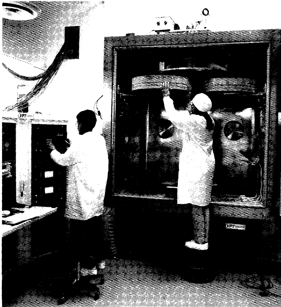
Jennifer Traylor and Roman Chrzan, specialists in the Optical Manufacturing Group, monitor application of dielectric thin films on optical elements in the newly installed 72-in. vacuum chamber. This chamber complements two other vacuum chambers in the Optical Manufacturing Department, which will be used to apply optical coatings to the OMEGA Upgrade mirrors, beamsplitters, and polarizers. The 72-in. chamber will be used to coat the largest of the optical components, including the frequency-conversion polarizers and ultraviolet transport mirrors.
