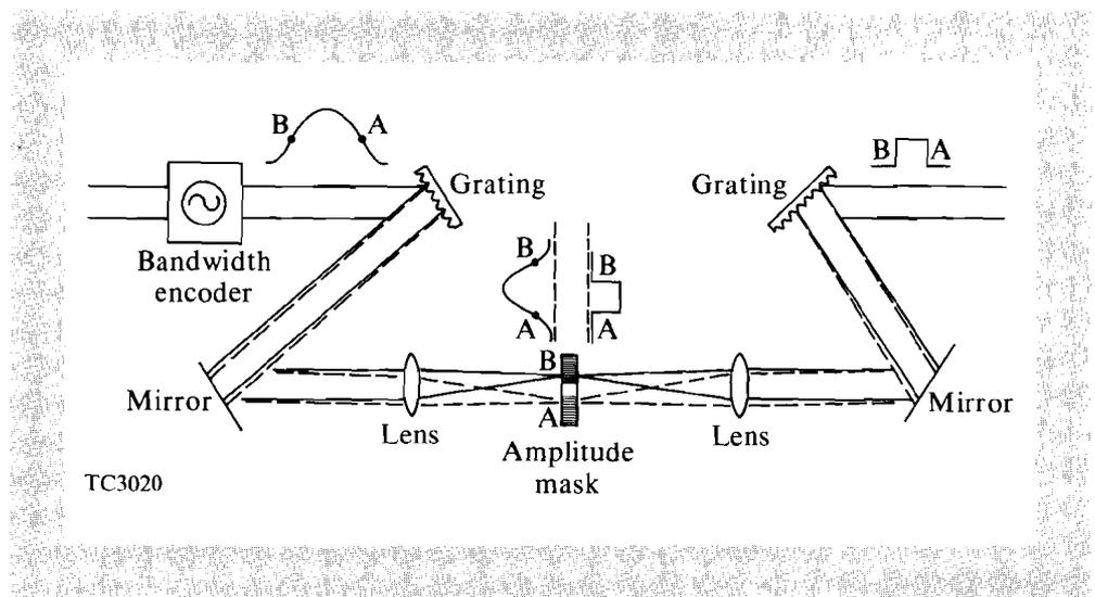
After the spectral encoding and filtration, the beam is recollimated with a lens and the spectral dispersion is removed with a second grating. At this point, temporal pulse shaping has been achieved. In general, only a small fraction of the encoded bandwidth has been used to shape the pulse, and the remainder is still in the form of phase modulation. The following options are available for continued manipulation of the beam:
