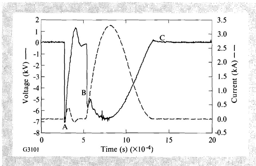
Fig. 48.15 Current and voltage for the prototype disk amplifier at 13.4-kV charging voltage.
