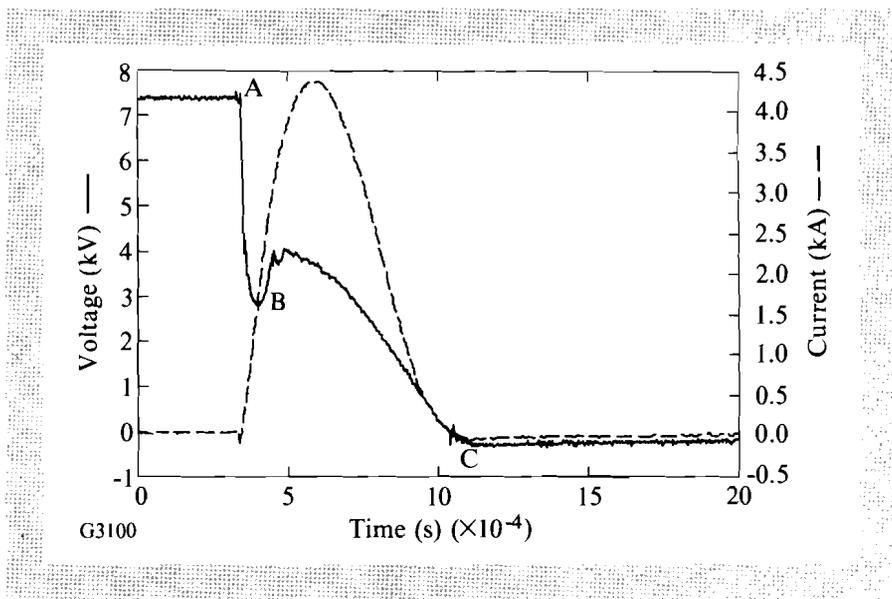
Fig. 48.14 Current and voltage versus time for the 90-mm-rod amplifier at 7.4-kV charging voltage.
