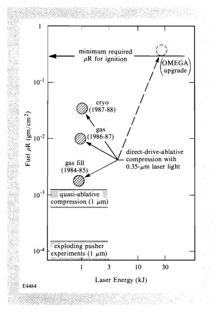
techniques. These experiments were the result of an intensive effort, which included (a) improvements of the target surface distribution of laser irradiation on the OMEGA laser; (b) the development and implementation of a new class of diagnostic instrumentation to measure high-density implosions; and (c) the implementation of cryogenic fuel-layer technology on the OMEGA facility. The results of these experiments were validated by a DOE-selected panel of scientists from other ICF laboratories.
