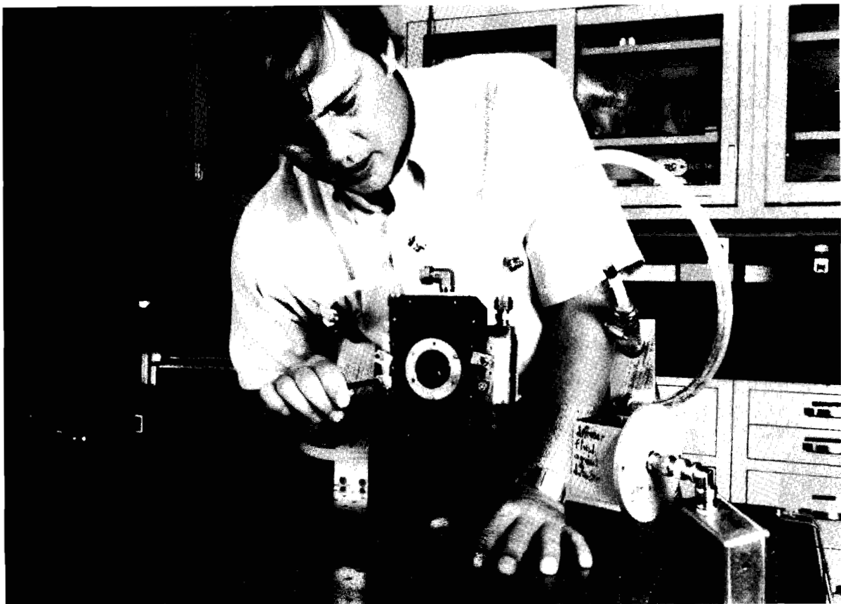
David Smith, an engineer in the high-repetition-rate, solid-state sources group, has been responsible for a large part of the design and development of the Cr:Nd:GSGG active mirror, which he is shown adjusting. The high-repetition-rate sources group is currently developing slab and active-mirror geometry amplifiers in both glass and crystalline media.
