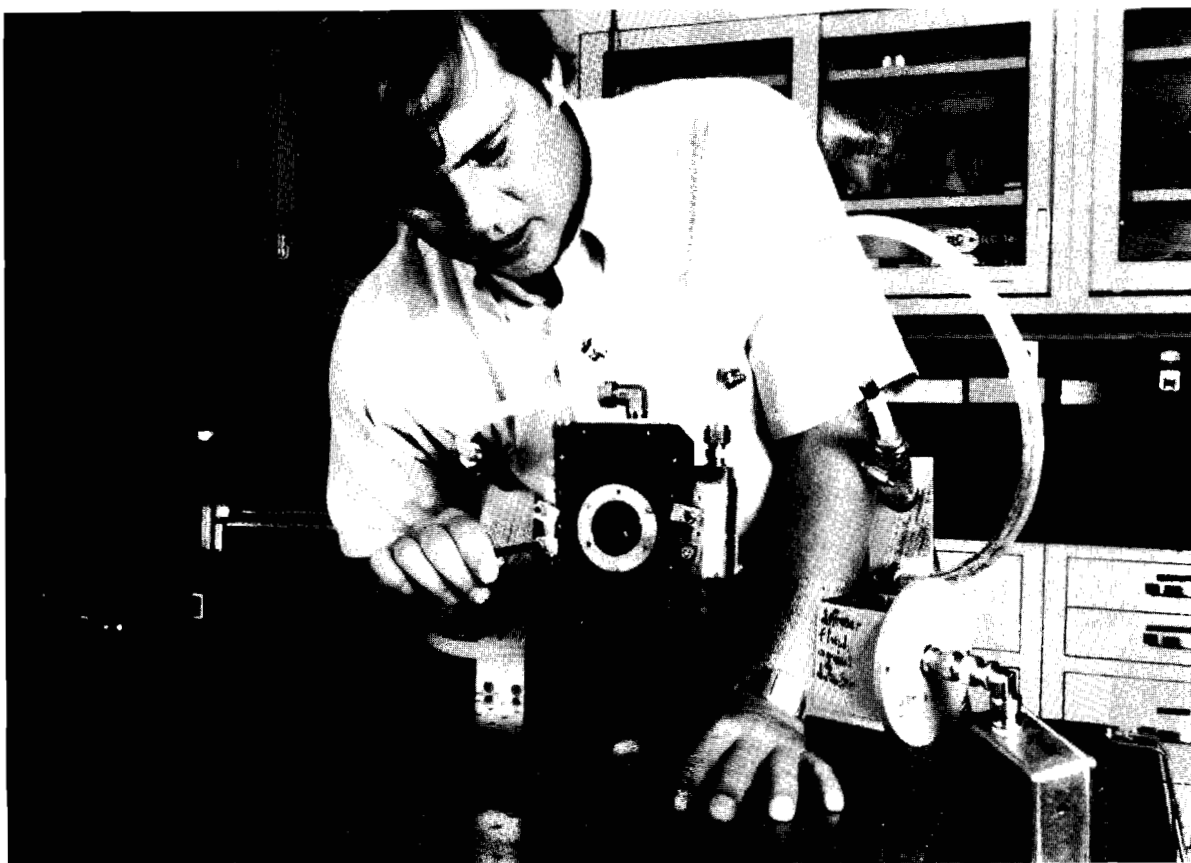
David Smith, an engineer in the high-repetition-rate, solid-state sources group, has been responsible for a large part of the design and development of the Cr:Nd:GSGG active mirror, which he is shown adjusting. The high-repetition-rate sources group is currently developing slab and active-mirror geometry amplifiers in both glass and crystalline media.
