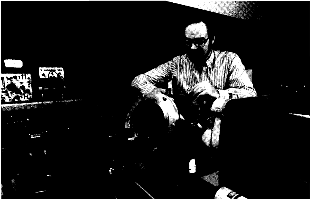
Roger Gram, a senior technical associate in the Target Fabrication Group, prepares a chamber for coating targets with plastic ablation layers. The targets are coated while they are being bounced in order to avoid the asymmetry introduced by a supporting stalk.
