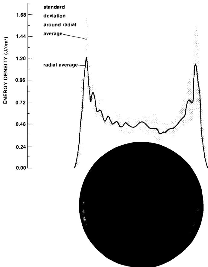
Figure 6 Near field beam profile for high energy, long pulse shot on OMEGA (shot 3606).
