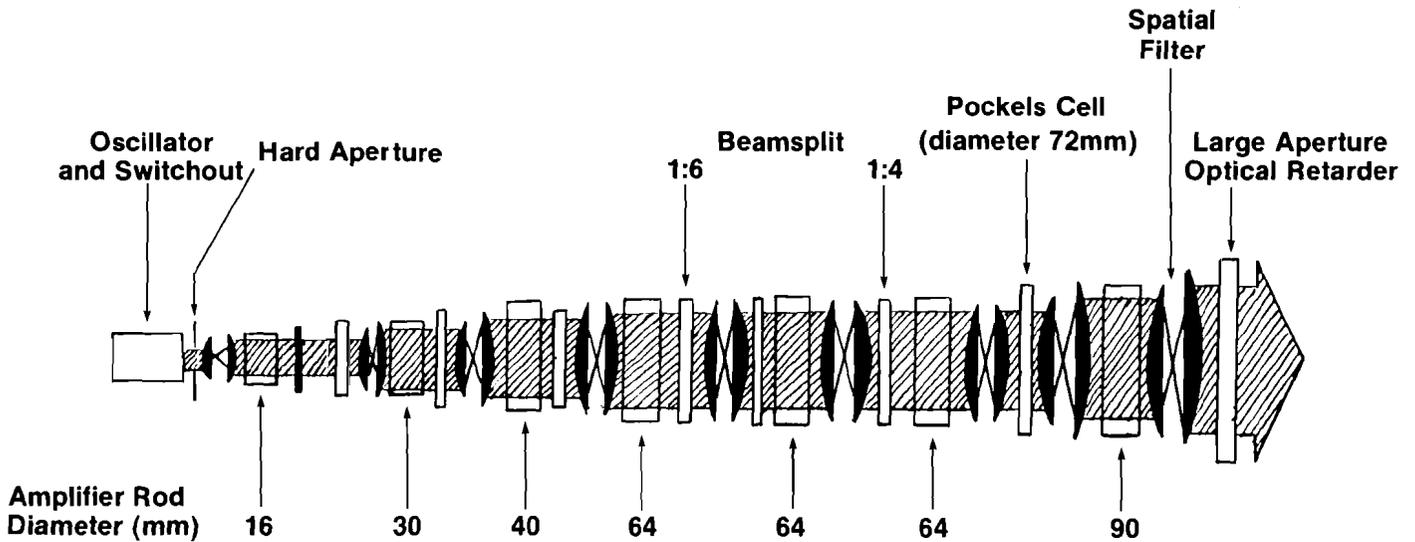
Figure 3 Staging diagram for OMEGA beamline.
