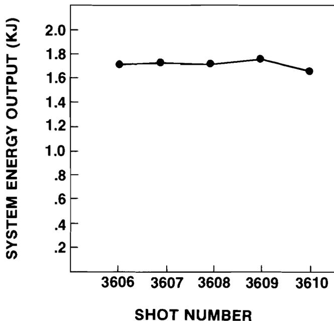
Figure 4 OMEGA energy output on long pulse series ( $264 \pm 15$  psec FWHM).
