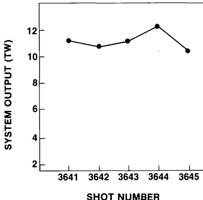
Figure 5 OMEGA power output on short pulse series ( $55 \pm 5$  psec FWHM).
