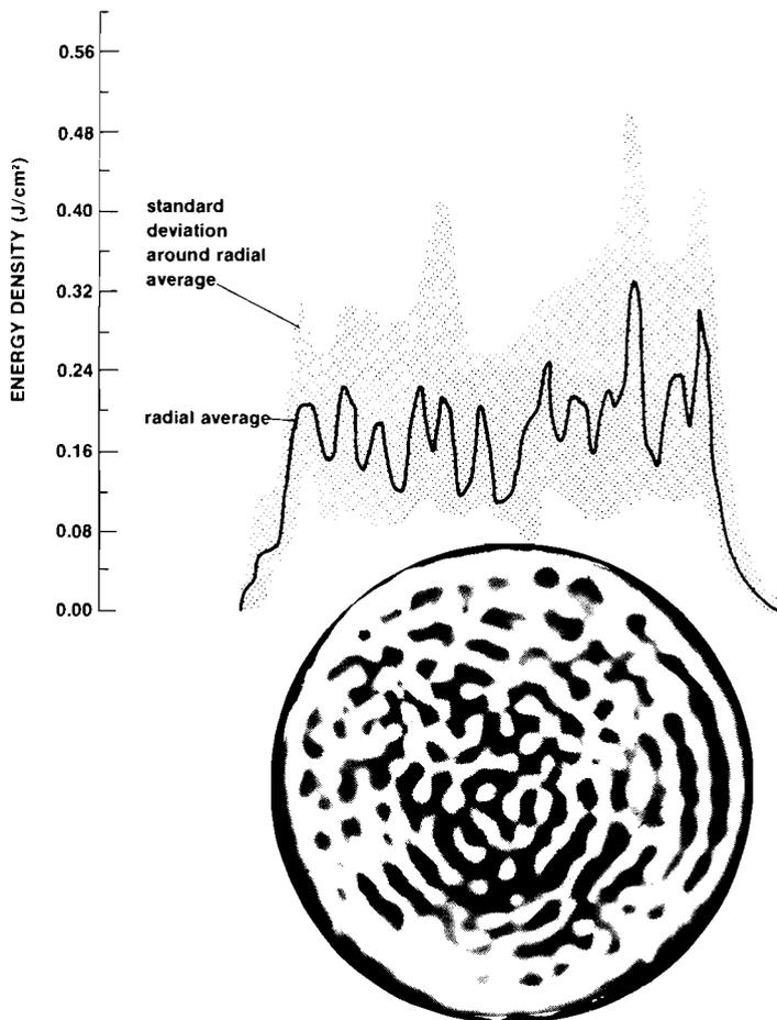
Figure 7 Near field beam profile for high power, short pulse shot on OMEGA (shot 3645).
