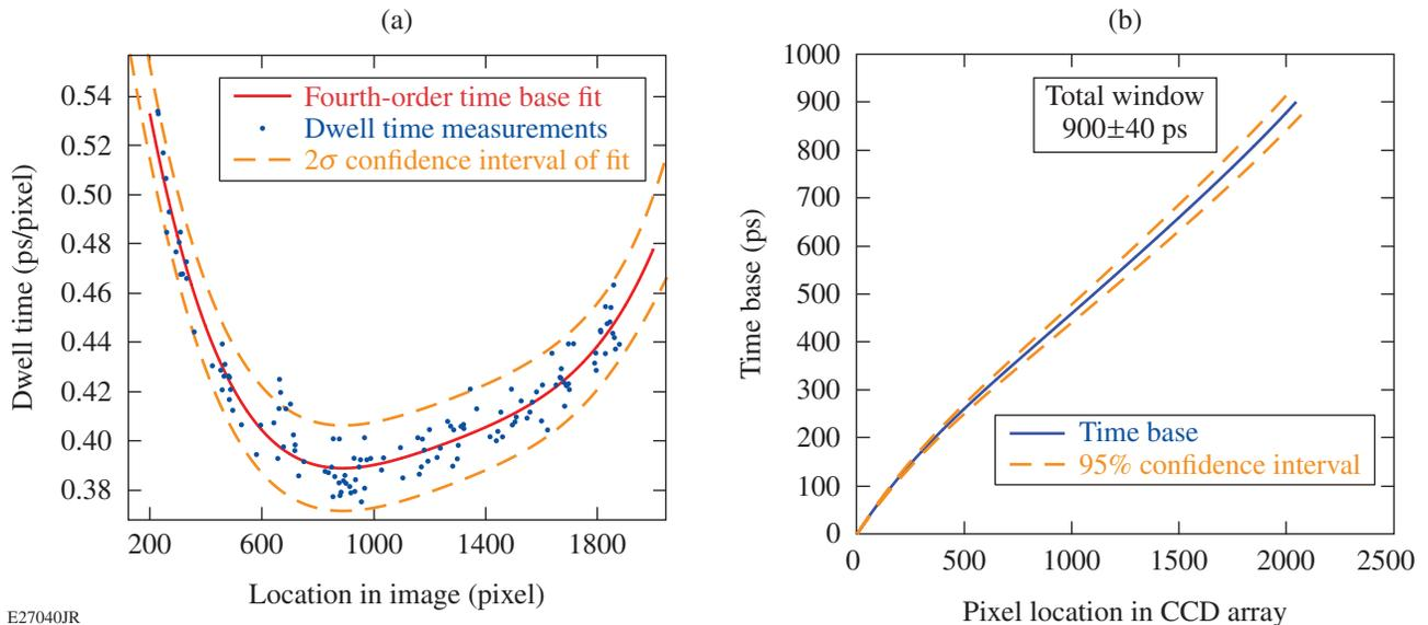
Figure 153.22 (a) The dwell time per pixel as a function of pixel location on the sweep window for the camera using the fast pulser; (b) the camera time base as a function of position on the CCD array.
