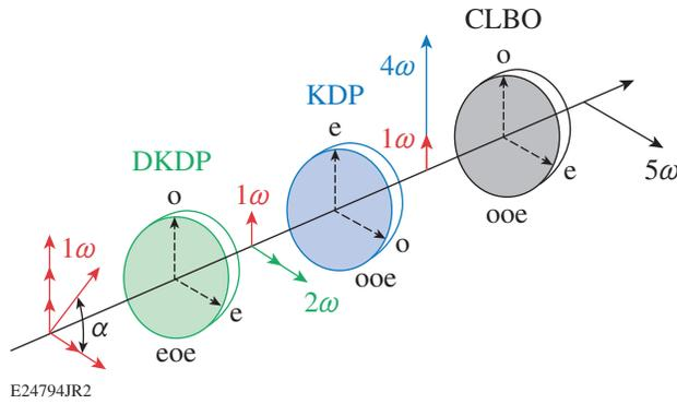
Figure 153.12 Schematic showing the orientation of the crystal axes and polarizations. The angle ( $\alpha$ ) of the  $1\omega$  polarization was set using a HWP for optimal conversion. e: extraordinary; o: ordinary.
