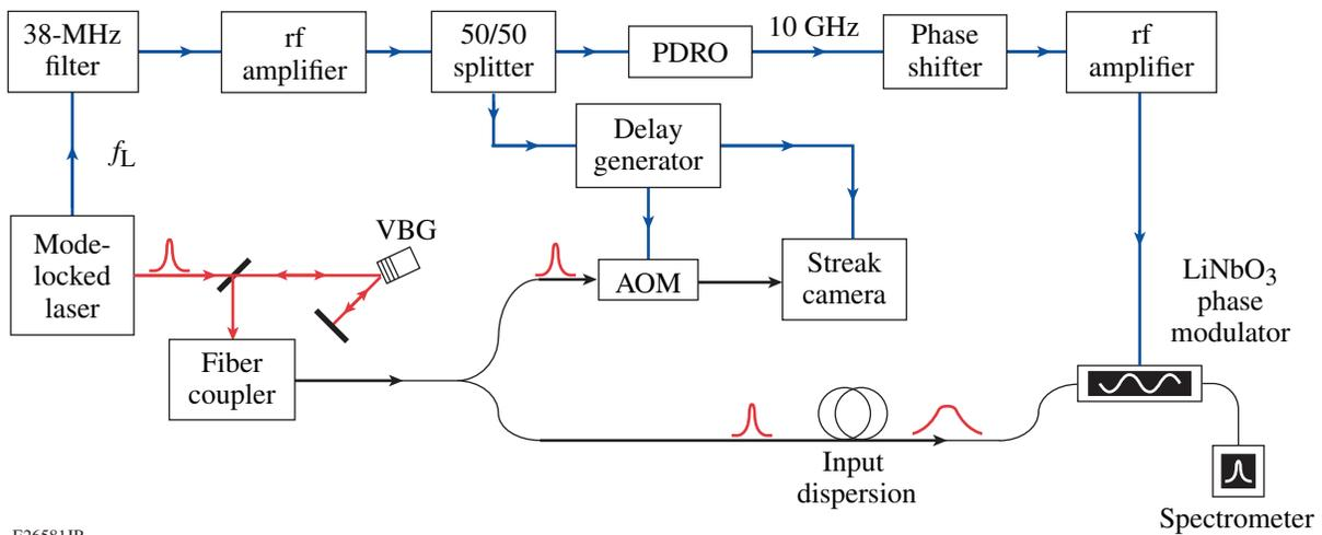
Figure 152.15 Experimental setup for a time-to-frequency converter using a phase modulator as a time lens and an optical fiber for the input dispersion. AOM: acousto-optic modulator; PDRO: phase-locked dielectric resonator oscillator; rf: radio frequency; VBG: volume Bragg grating.
