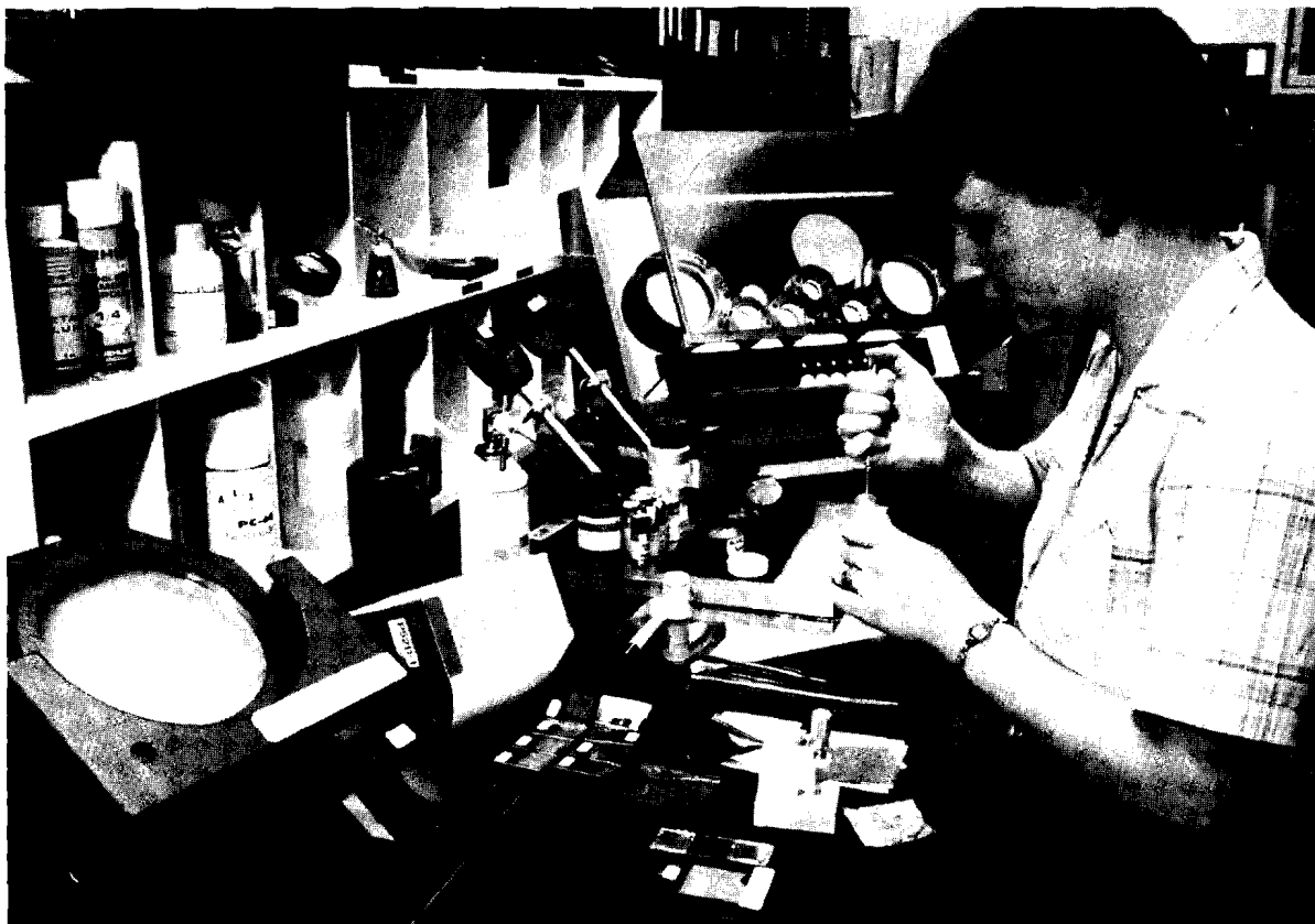
Laboratory Engineer Kathy Cerqua, of the Optical Materials Group, is shown fabricating a liquid-crystal circular polarizer. The Laboratory for Laser Energetics is carrying out research on the use of liquid-crystal devices in a number of high-power laser applications.
