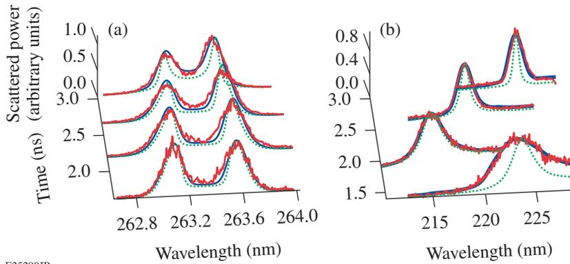
Figure 147.20 Measured spectral lineouts (red) and the corresponding calculated spectra (blue) at several different times for the (a) IAW and (b) EPW collected at 400 μm from the initial target surface. The green dotted curves correspond to calculated spectra using the same plasma parameters as the best-fit curve (blue) but without including gradient/wave-vector effects.
