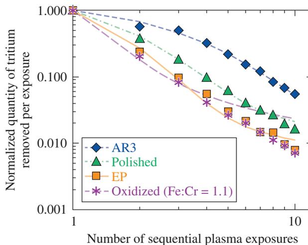
Figure 147.52 Comparison of the results obtained from pulsed-plasma experiments to best fits (calculated using QTRIMM) of various samples charged with tritium in Batch B. The error in each data point is  $\pm 5\%$ .
