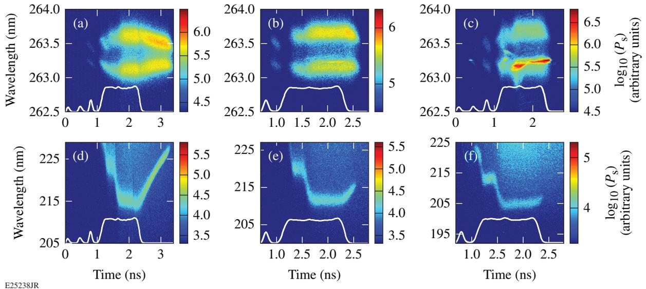
Figure 147.17 Thomson scattering from [(a)–(c)] IAW's and [(d)–(f)] EPW's at [(a),(d)] 400  $\mu\text{m}$ , [(b),(e)] 300  $\mu\text{m}$ , and [(c),(f)] 200  $\mu\text{m}$  from the initial target surface. The drive-laser pulse shape is overlaid. The bright features at  $\sim 263.2$  nm in the IAW spectra correspond to reflected or refracted light from the probe beam.
