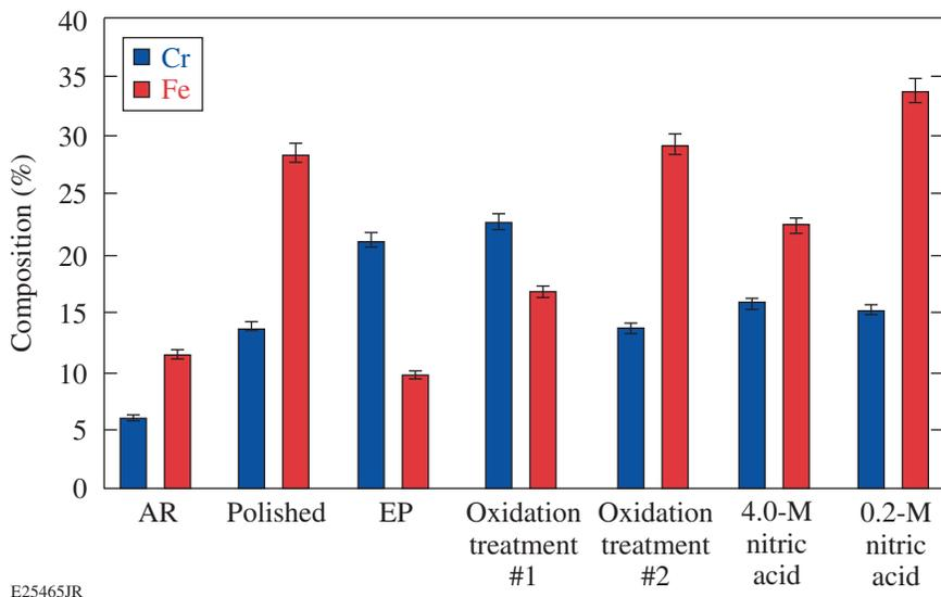
Figure 147.44 Measured Cr and Fe content in select samples using x-ray photoelectron spectroscopy (XPS).
