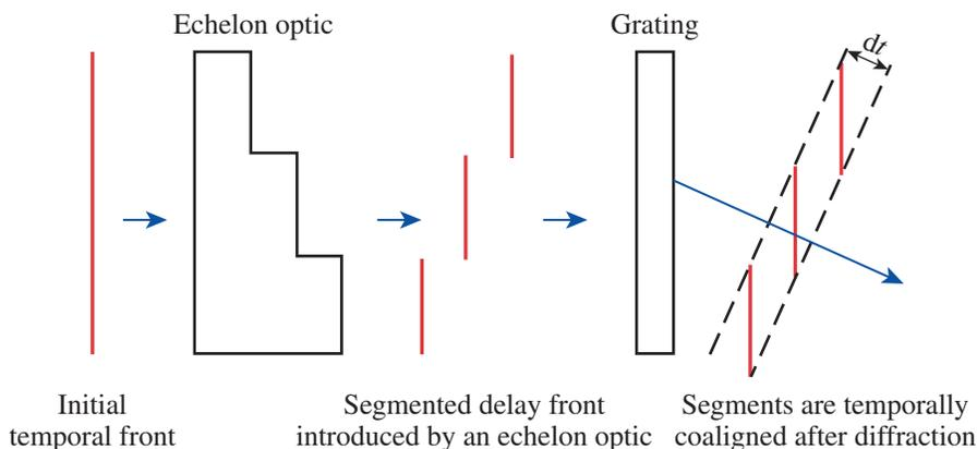
Figure 147.36 PFT can be reduced with no loss to throughput by segmenting the incoming beam into multiple sub-elements that are individually delayed to compensate for the path-length difference introduced by the diffraction grating. The residual PFT is limited to the accumulation across a single segment and the overall temporal resolution is improved by a factor equal to the number of sub-elements used.
