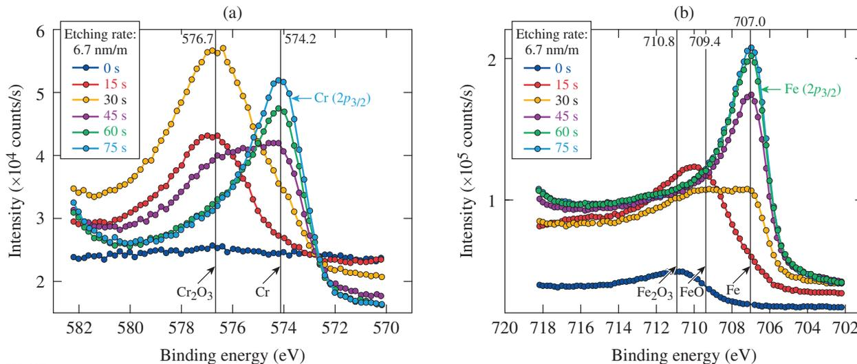
Figure 147.45 XPS photoelectron spectra for (a) Cr and (b) Fe atoms bound to the surface of as-received (AR) samples.
