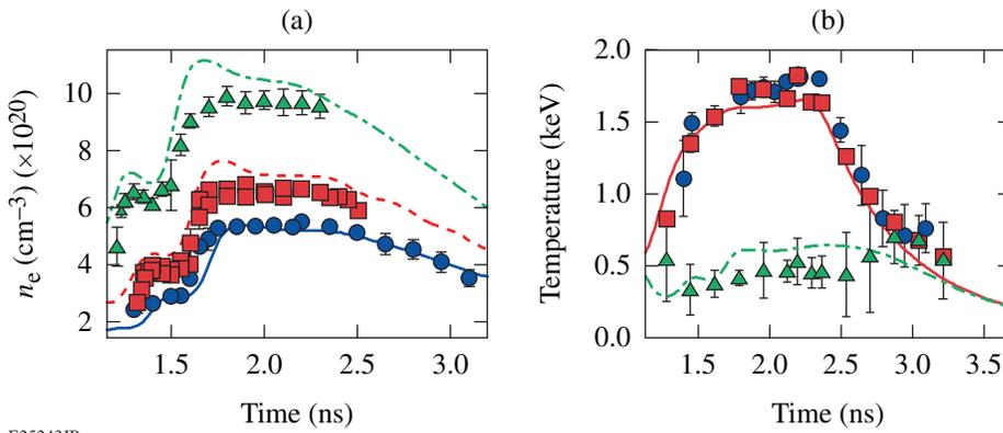
Figure 147.21 (a) Measured (symbols) and simulated (curves) electron density at 400 μm (circles), 300 μm (squares), and 200 μm (triangles) from the initial target surface. (b) Electron temperature inferred from IAW (squares) and EPW (circles) spectra, and ion temperature (triangles) inferred from the IAW spectra at 400 μm. The error in absolute timing is ~100 ps.
