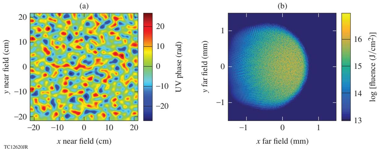
Figure 146.19 The intermediate NIF polar-direct-drive (PDD) distributed phase plate (DPP) design crafted for (a) an equatorial beam profile and (b) the resultant speckled spot. The speckled image on the log scale demonstrates the remarkable speckle rejection and smooth profile at low intensity not obtainable using other methods. Note that the design objective function and the extracted envelope are nearly indistinguishable at a <1% rms (root-mean-square) error.
